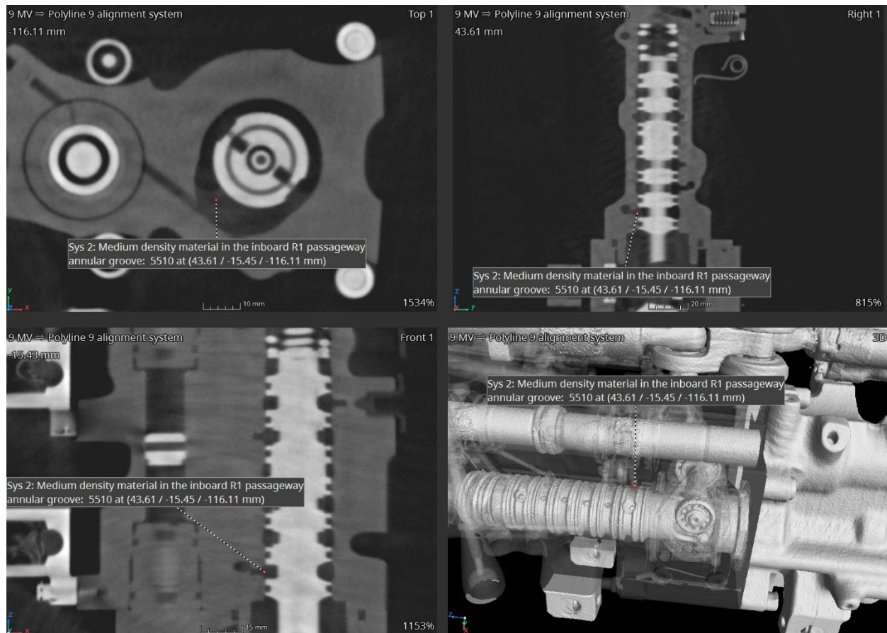
Figure 28. CT images of System 2 portion of yaw ILCA illustrating medium density material in the inboard R1 passageway annular groove between the sleeve and housing. (9MV)
