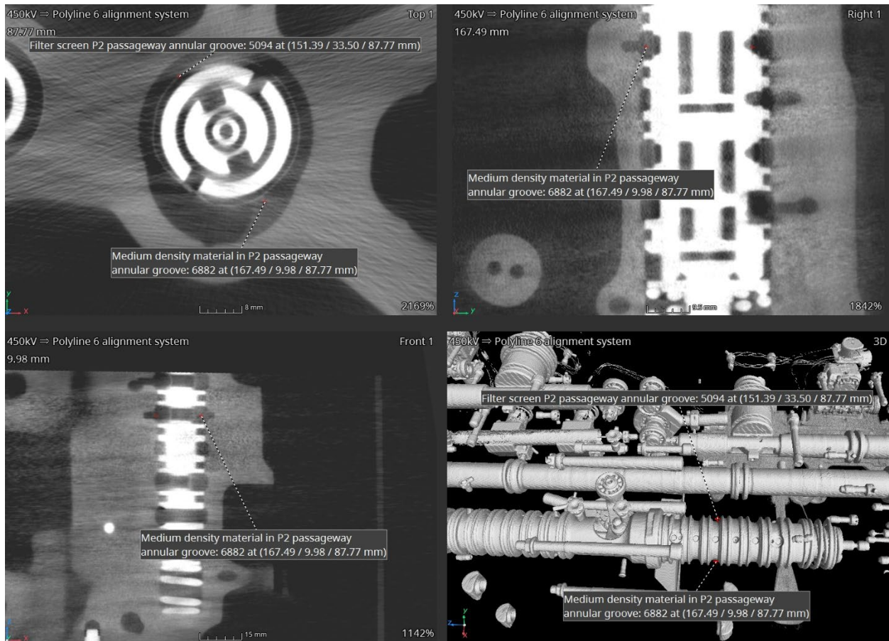
Figure 14. CT images of System 1 portion of the yaw ILCA illustrating medium density material and the filter screen in the P2 passageway annular groove between the sleeve and housing. (450 kV)
