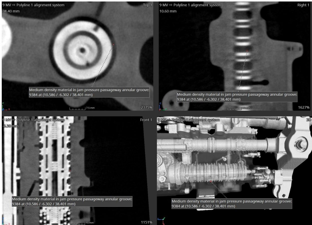
Figure 12. CT images of System 1 portion of yaw ILCA illustrating medium density material in jam pressure passageway annular groove between the sleeve and housing. (9 MV)
