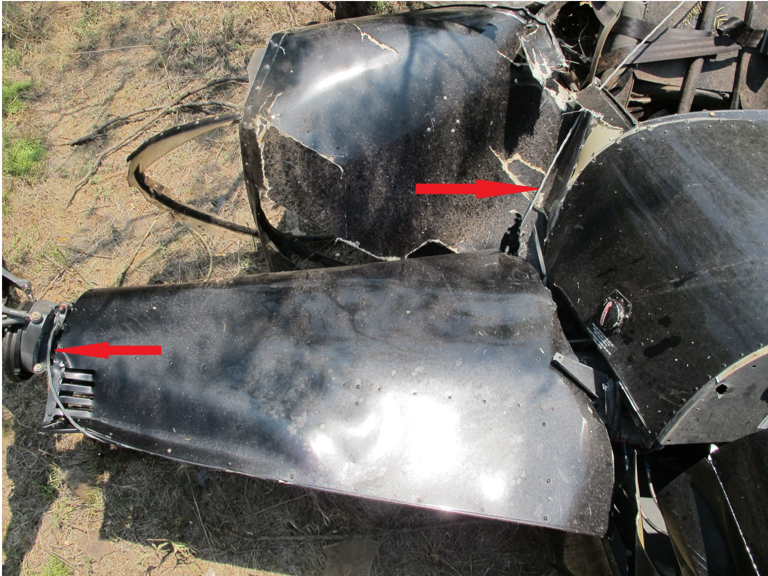
Photograph 4 - Wire Wrapped Around Swashplate and Lower Mast Fairing (Courtesy of NTSB)
