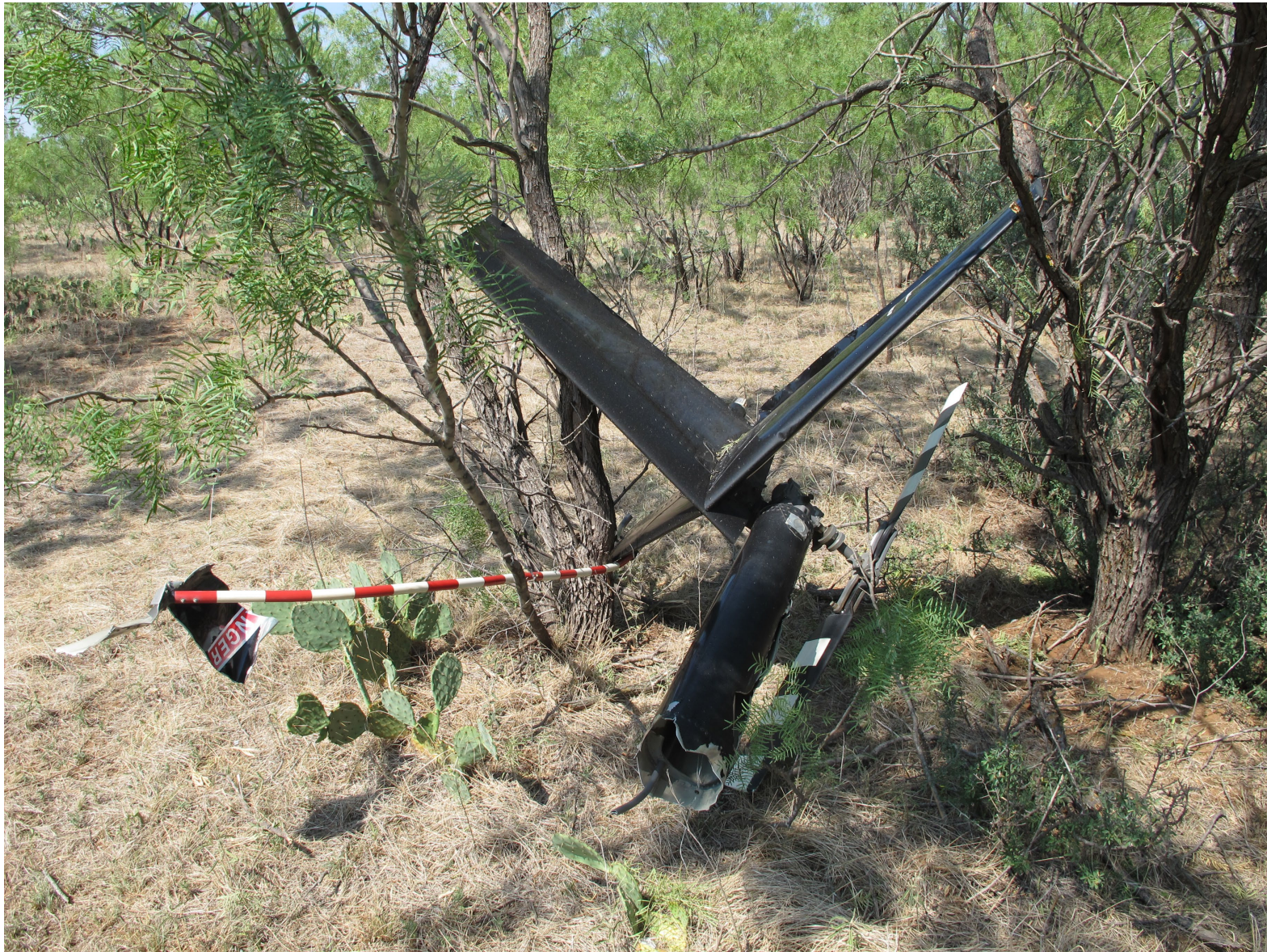
Photograph 2 - Separated Tail Rotor Section at Accident Site (Courtesy of NTSB)
