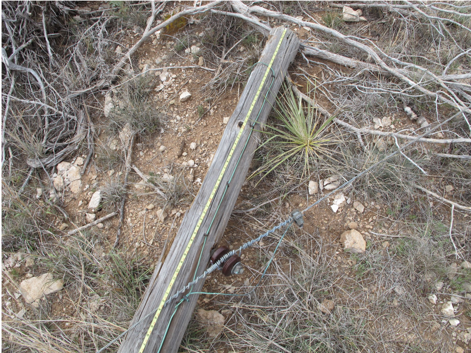
Photograph 7 - Broken Pole and Wire (Courtesy of NTSB)
