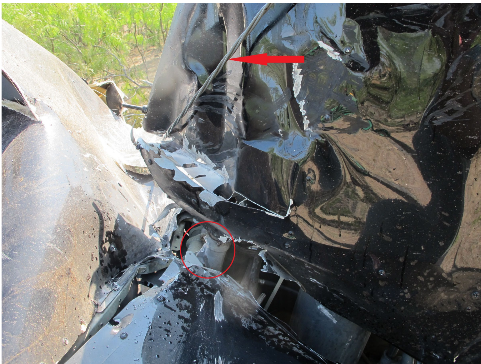
Photograph 3 - Wire Wrapped Around Swashplate and Mast Fairing (Courtesy of NTSB)
