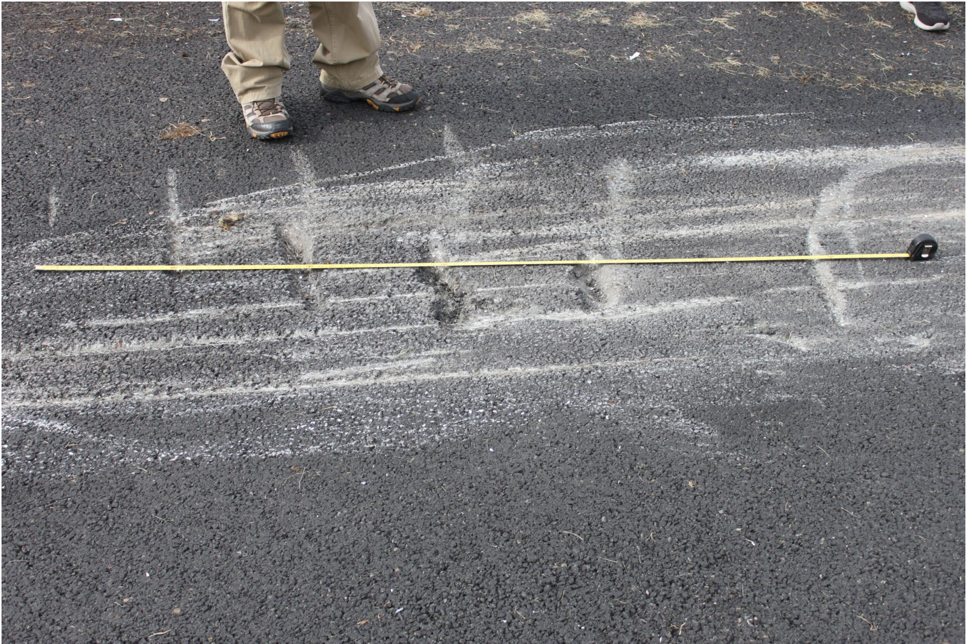
Photo 5 – Propeller Strike Marks at Accident Site
