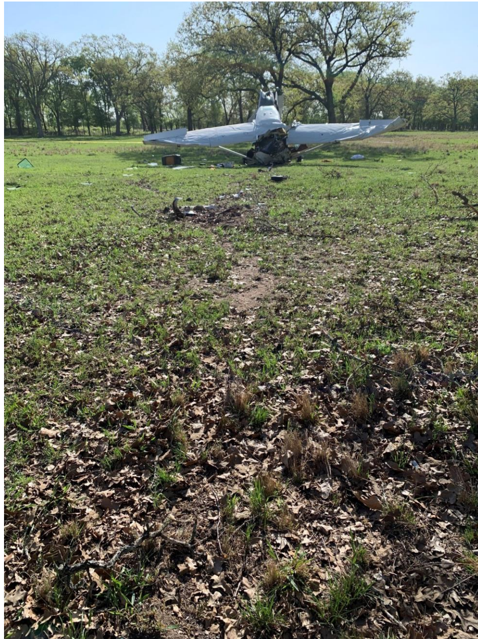
Photo 9 – Wings Witness Marks, and Debris Field
