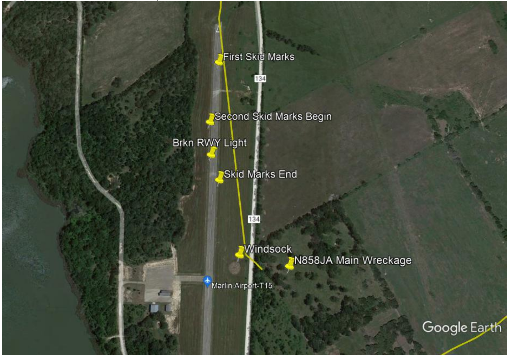
Runway Skid Marks and Accident Scene Locations, N858JA
