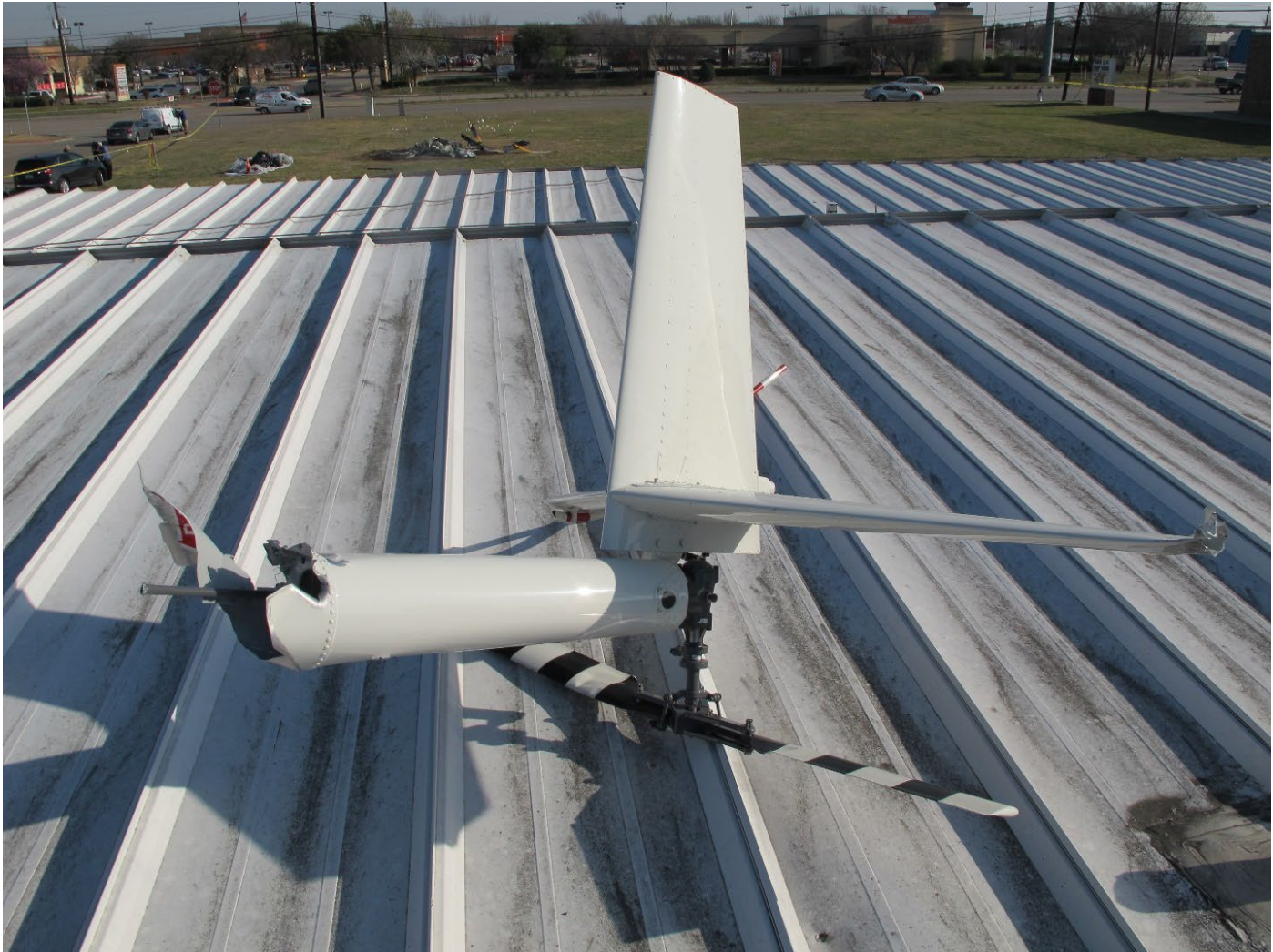
Portion of Tail Section with Tail rotor Assembly Still Attached. Main Wreckage in Background.
