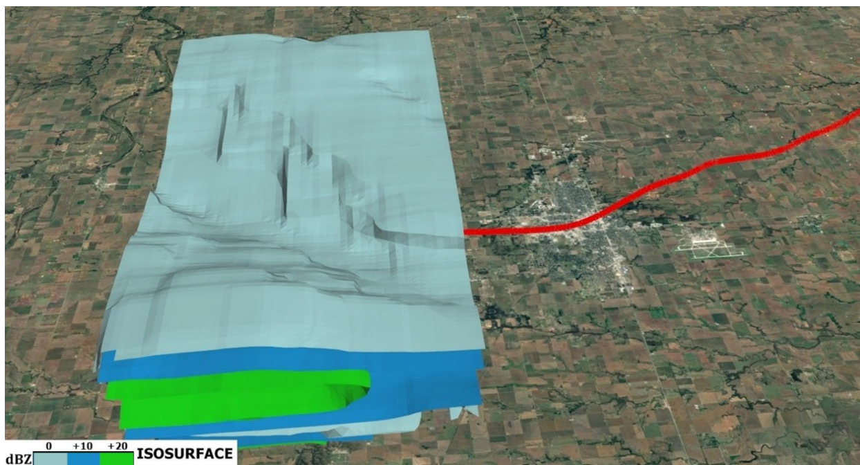
Figure 6 - Accident aircraft flight path with 3D 0, +10 and +20 dBZ isosurfaces overlaid.
