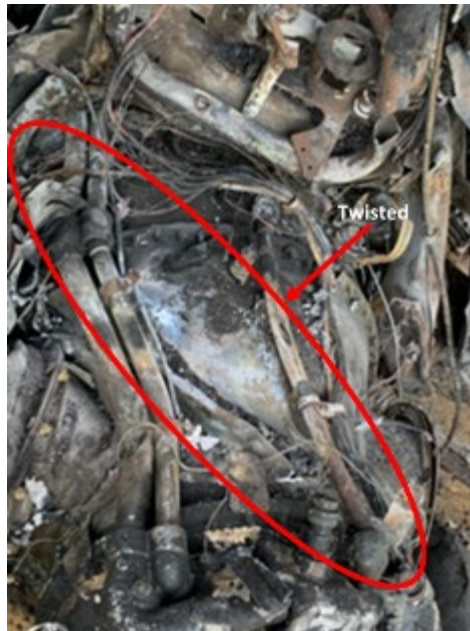
PHOTO 5: EXHAUST DUCT HOUSING TWIST
