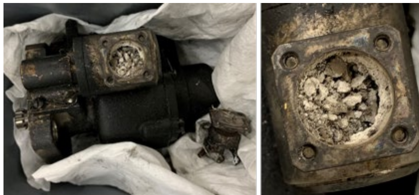
PHOTO 49: FEATHERING SOLENOID REMOVED FROM GOVERNOR (COURTESY OF WOODWARD).
