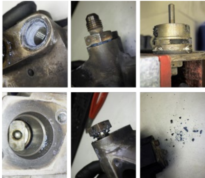
PHOTO 40: BRITTLE PACKINGS (COURTESY OF P&WC)
