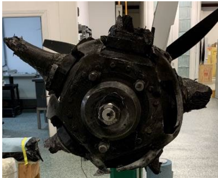
PHOTO 27: BURNED PROP HUB
