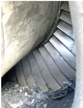
PHOTO 14: 2 ND STAGE PT BLADES, WITH CHARRED AIRFRAME DEBRIS (BOTTOM)
