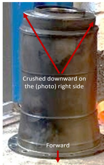
PHOTO 15: PT SHAFT HOUSING
