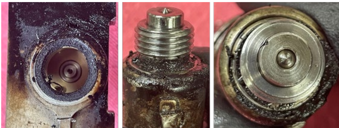
PHOTO 62: BURNT MATERIAL ON HOUSING, WITH THREADS & POPPET EXPOSED (COURTESY OF WOODWARD)
