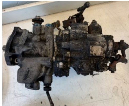
PHOTO 24: FUEL PUMP AND FUEL CONTROL UNIT
