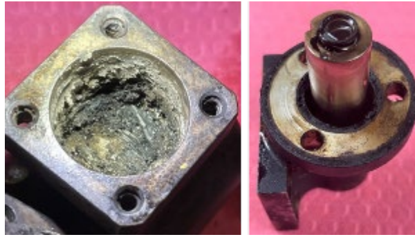
PHOTO 59: DEPOSITS IN THE HOUSING (LEFT) AND EXPOSED SPRING IN THE SLEEVE(COURTESY OF WOODWARD)
