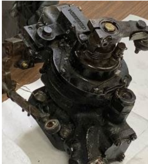
PHOTO 43: PROPELLER GOVERNOR, UNPACKED AT WOODWARD (COURTESY OF WOODWARD)
