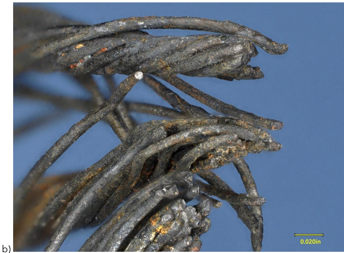
Figure 3. Images of the fractured upper cable: a) and b) fractured strands, as indicated in figure 1c.
