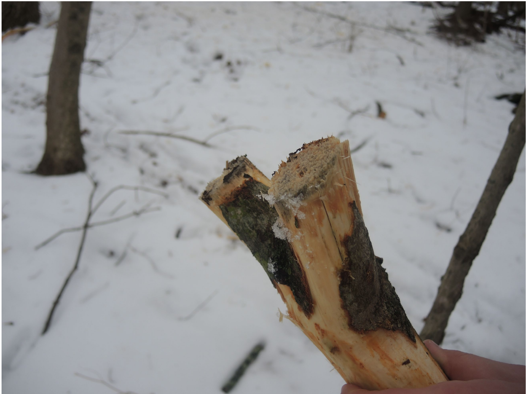
Photo 18 - Propeller Strike to Tree Branch (Source: NTSB)
