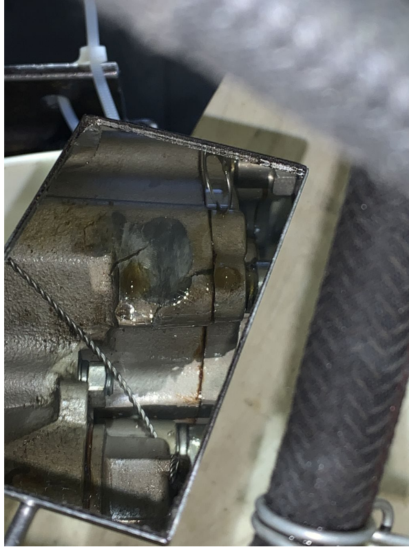
Figure 5 - Impact damage to oil filter housing
