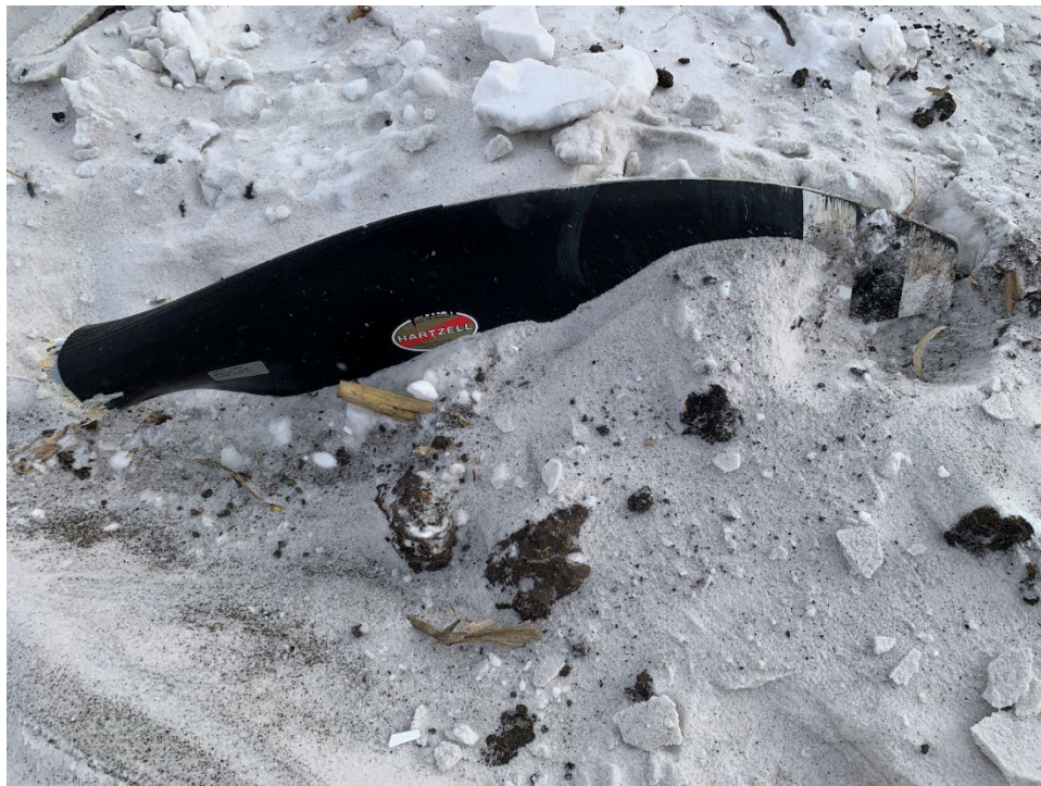
Figure 17: Propeller Blade at the First Identified Point of Impact
