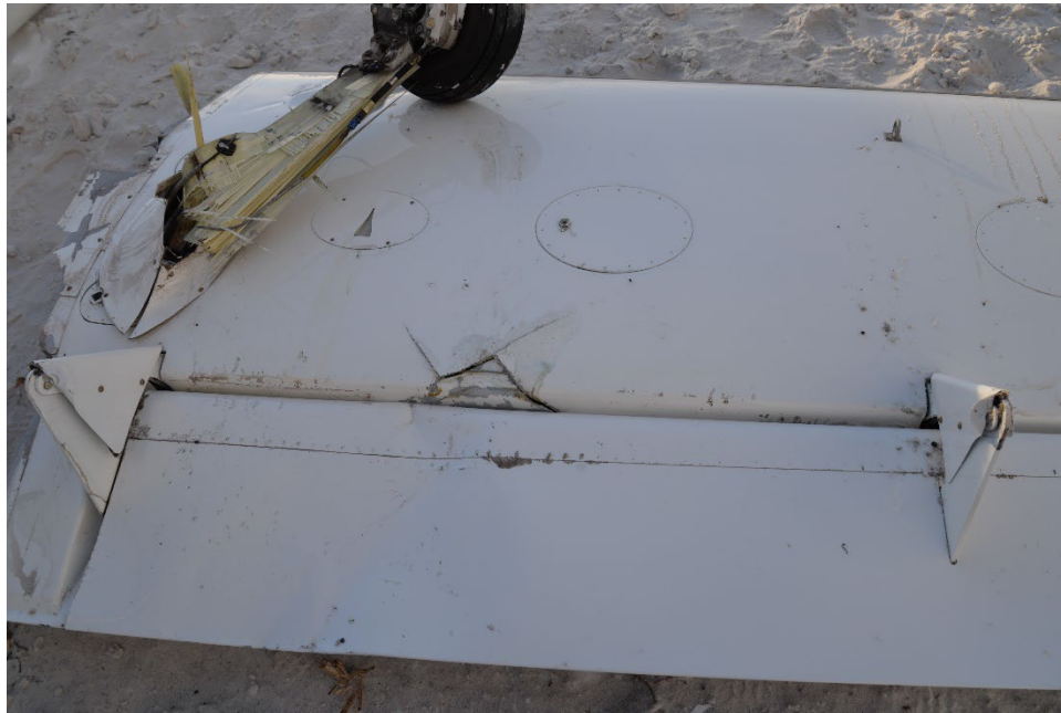
Figure 14: Underside inboard left wing. Note: blue staining.
