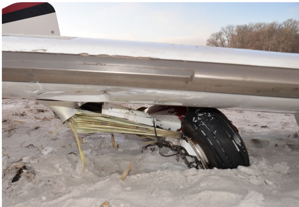
Figure 12: Splintered left Landing gear Strut
