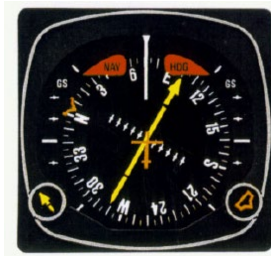
Photo 3: KI 525A Pictorial Navigation Indicator (Source: Bendix King Pilot's Guide)
