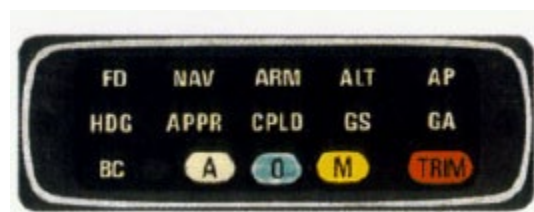
Photo 5: KA 285 Annunciator Panel (Source: Bendix King Pilot's Guide)
