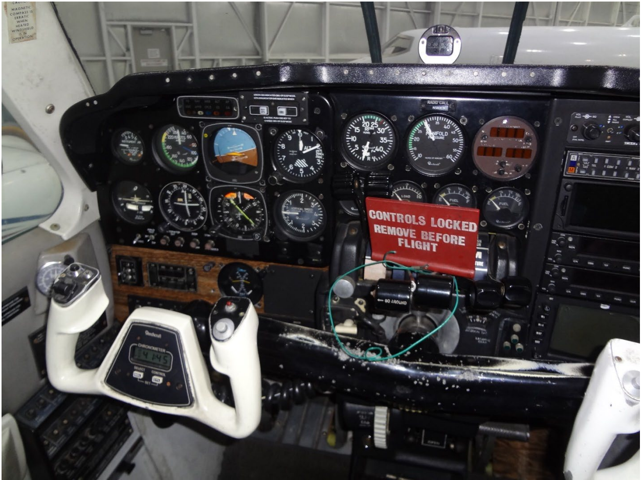
Photo 6: Instrument Panel of N583CK - Similar as the Accident Airplane (Note: Dual yoke was not on the accident airplane)
