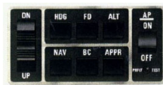
Photo 4: KC 290 Mode Controller (Source: Bendix King Pilot's Guide)
