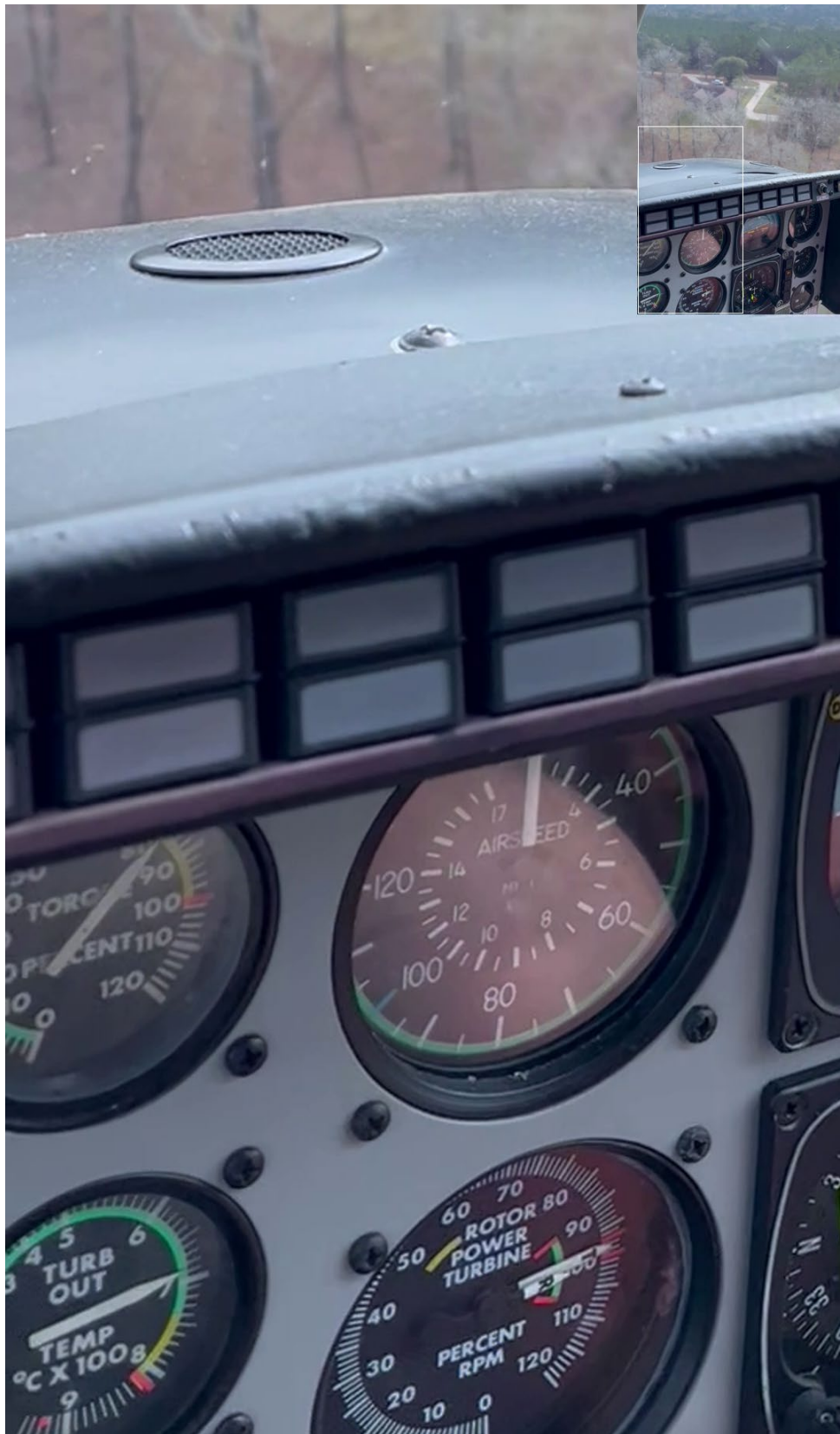
Figure 6. Zoomed in portion of the Torque and Turbine Outlet Temperature gauges captured at 0:38 Video Elapsed Time.
