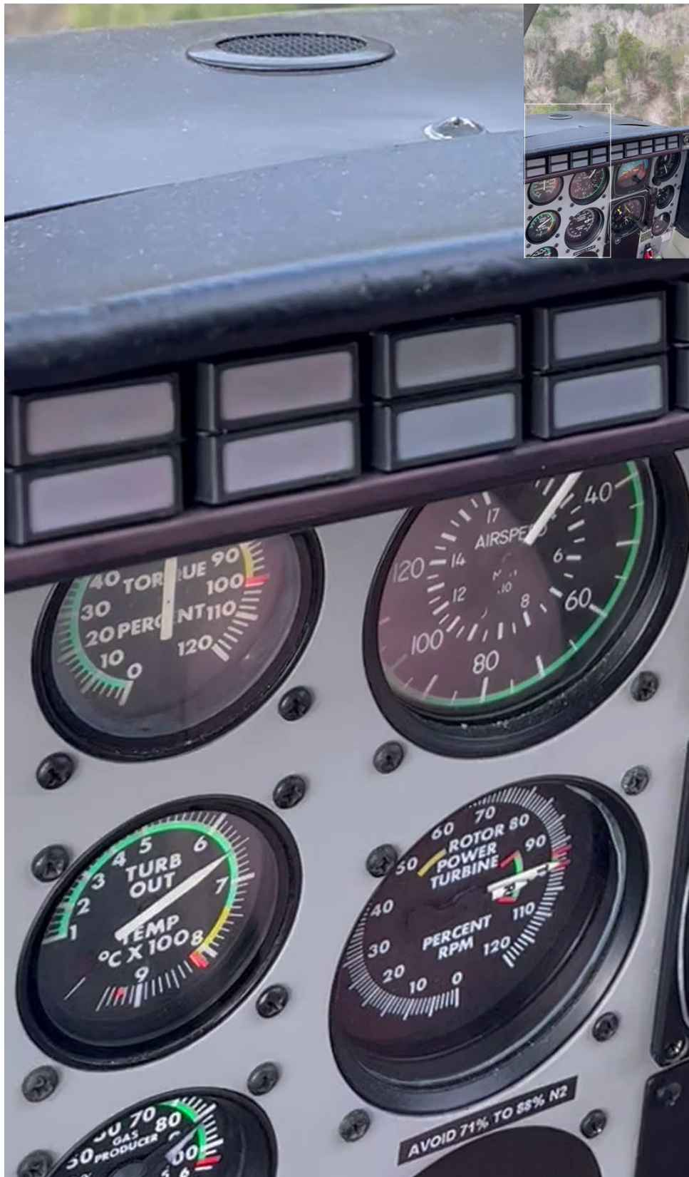
Figure 4. Zoomed in portion of the Torque and Turbine Outlet Temperature gauges captured at 0:26 Video Elapsed Time.
