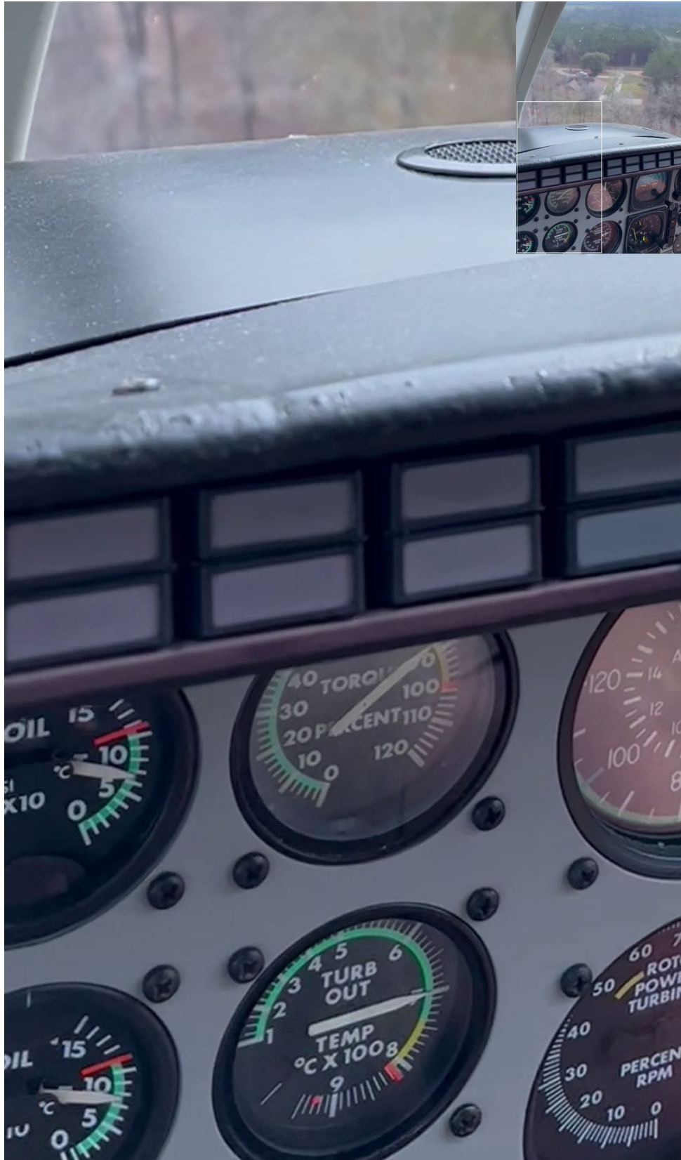
Figure 7. Zoomed in portion of the Torque and Turbine Outlet Temperature gauges captured at 0:39 Video Elapsed Time.
