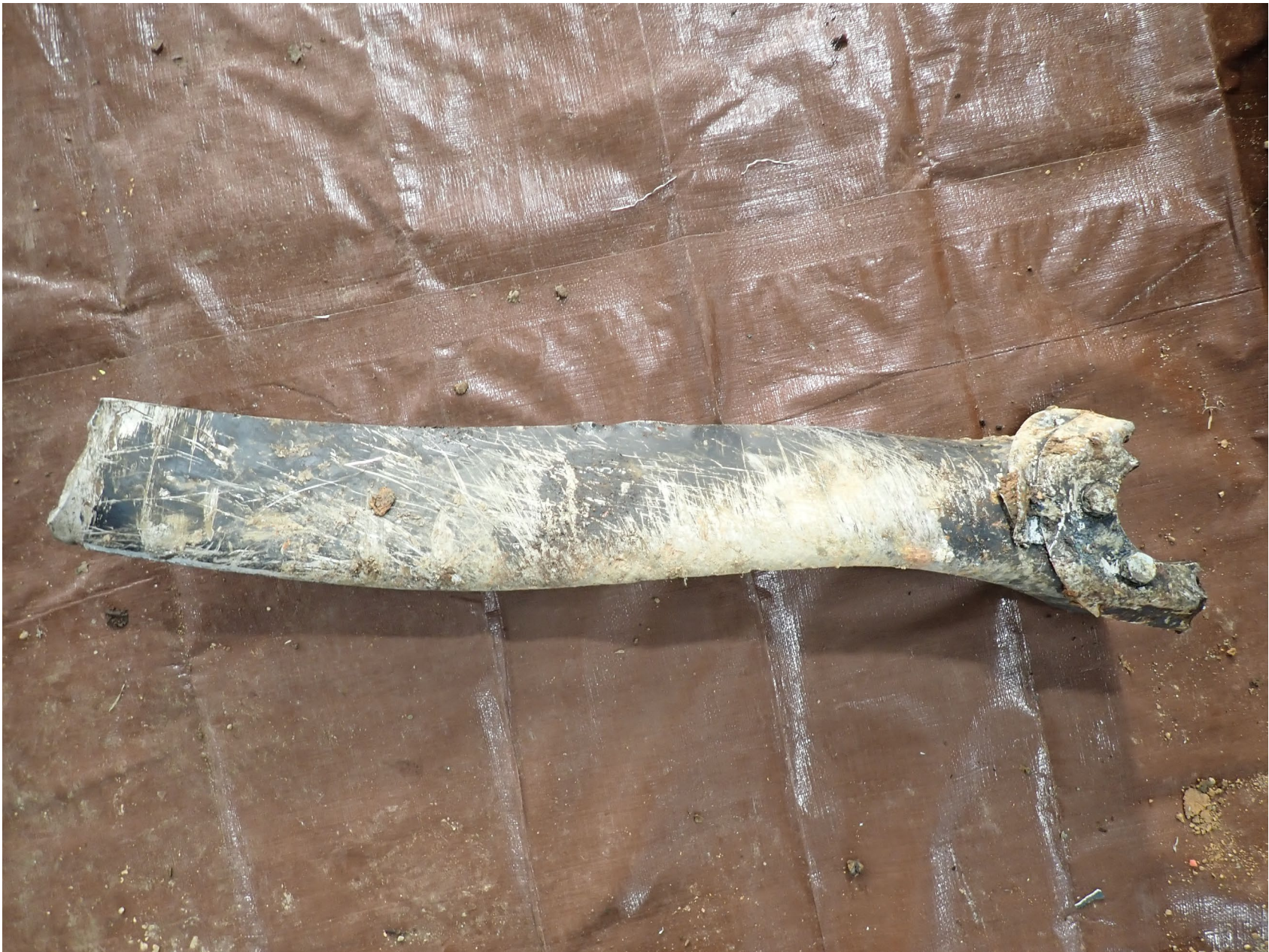
Photo 10 – View of propeller blade B at the salvage facility (courtesy of Textron Aviation).
