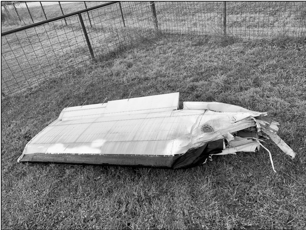
Figure 2. Outboard section of Cessna 208B right wing
