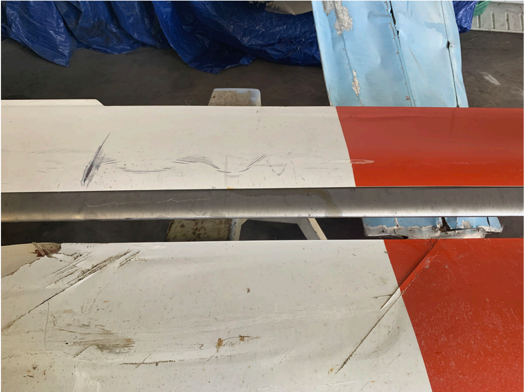
Photo 2 – Braided Cable Mark – Red Blade
