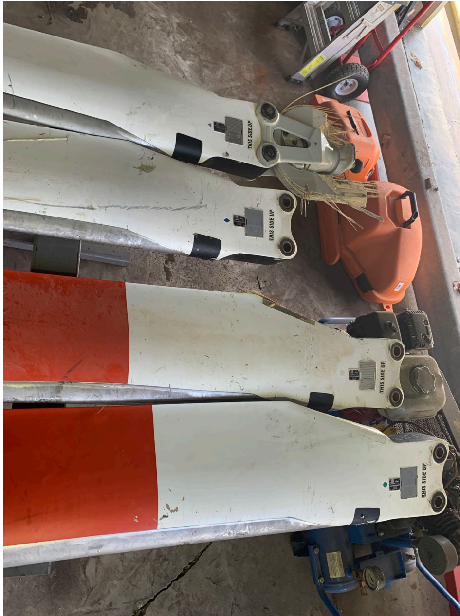
Photo 3 – Braided Cable Mark – Blue Blade – Second From Top
