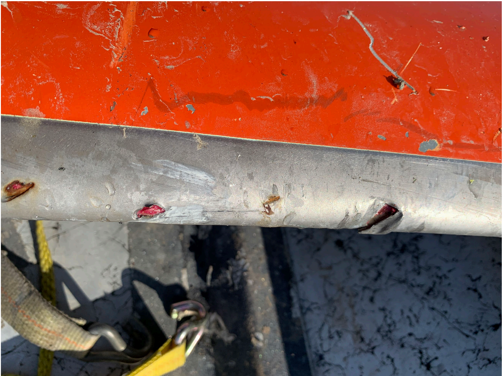
Photo 4 – Blue Blade Leading Edge Marks
