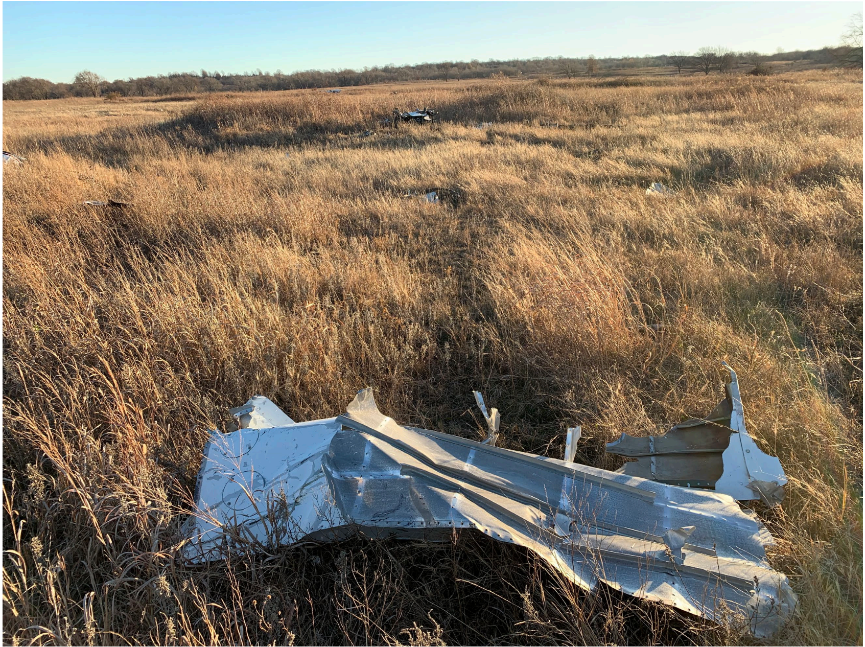
Photo 3 – Separated wing structure
