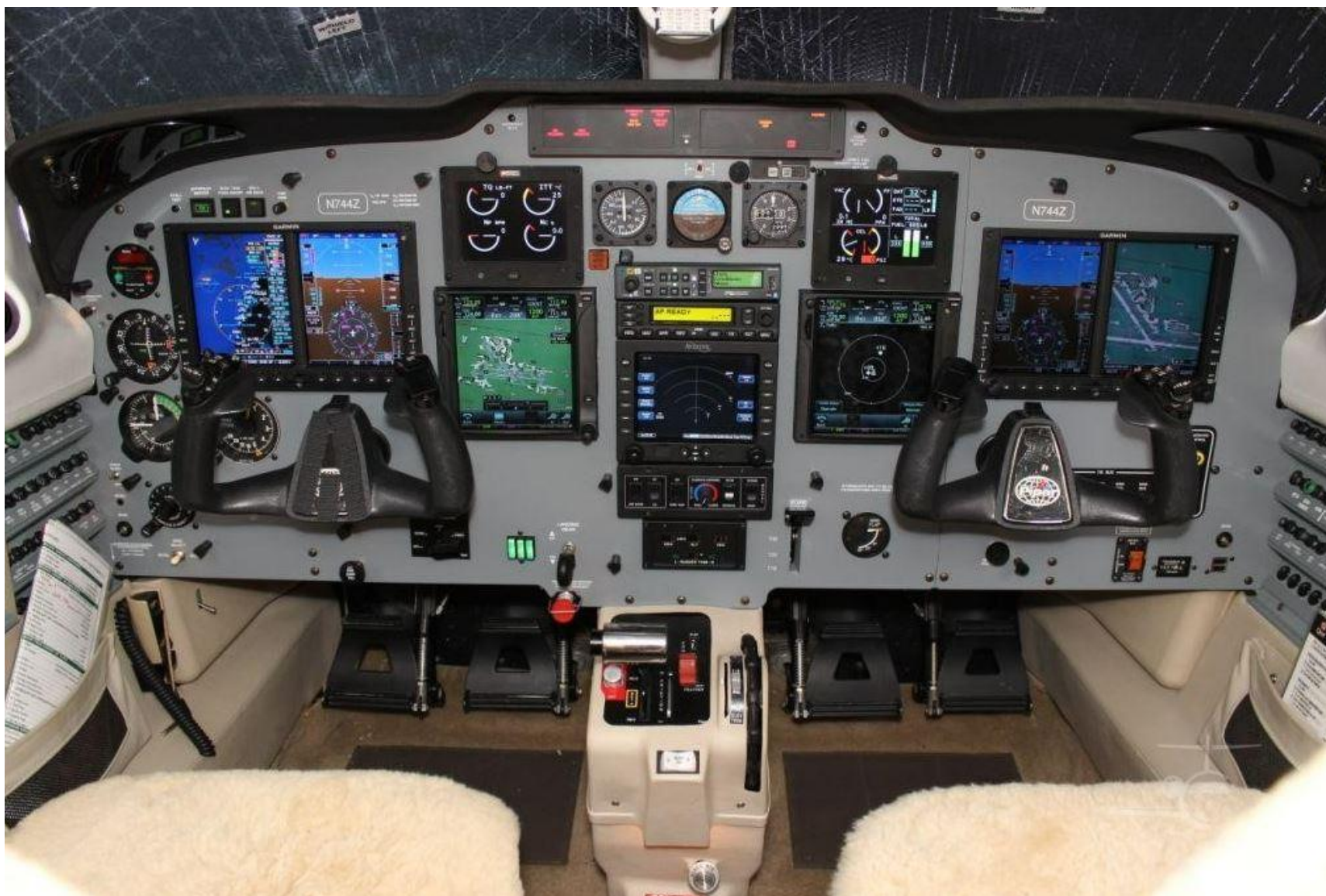
Figure 23. The instrument panel of N744Z. The photo was taken from an online sales posting for the accident aircraft was undated. The sales listing advertised "New dual Garmin 500 glass package New pilot side synthetic vision."
