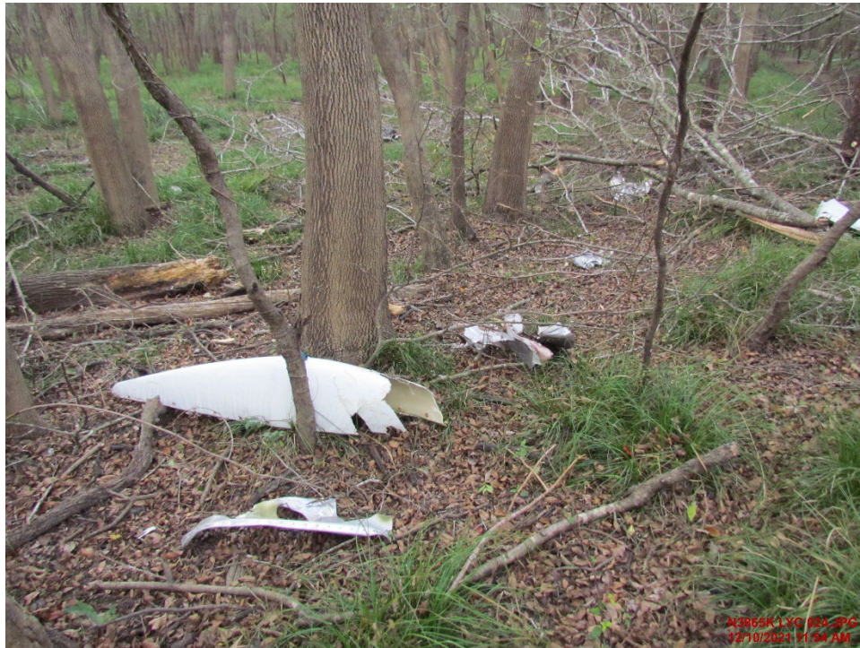
Figure 4: Fragments of Right Wing Scattered Below Topped Trees
