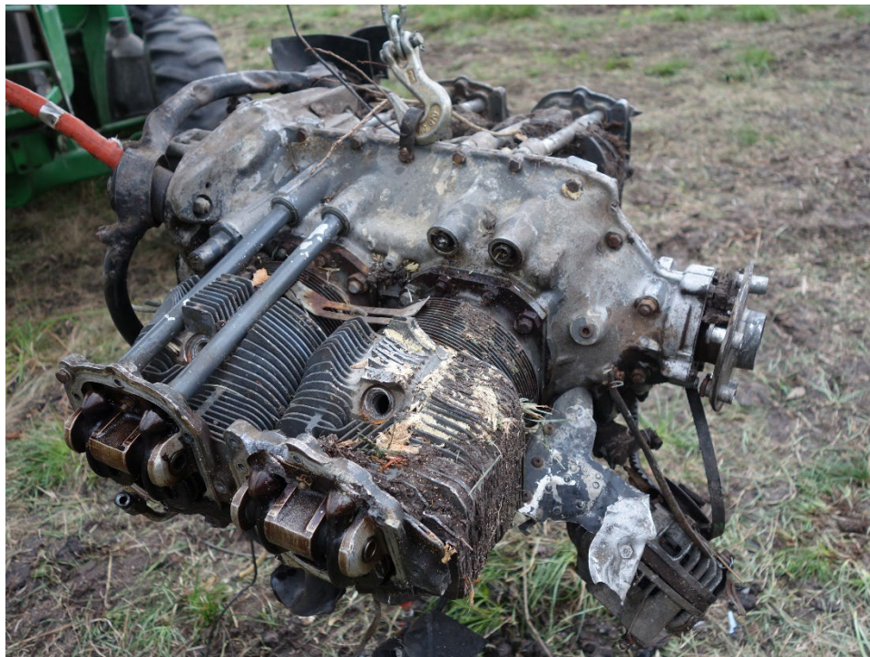
Figure 22: Damage to Number 1 Cylinder
