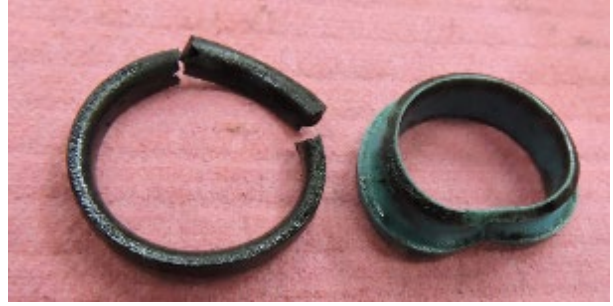
Figure 8. Seal 6, scraper seal removed from the end gland.
