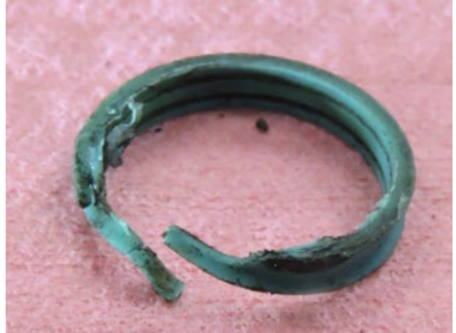
Figure 13. Seal 2, primary seal, Teflon portion.
