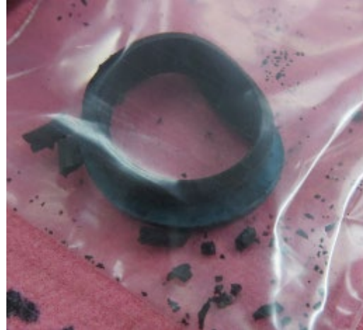
Figure 16. Scraper seal, seal 6. Teflon scraper and pieces of carbonized o-ring.
