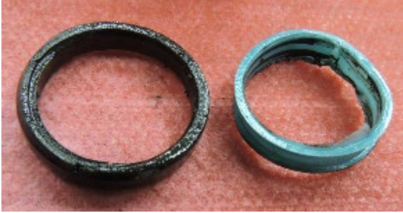
Figure 7. Seal 5, primary seal removed from the end gland.
