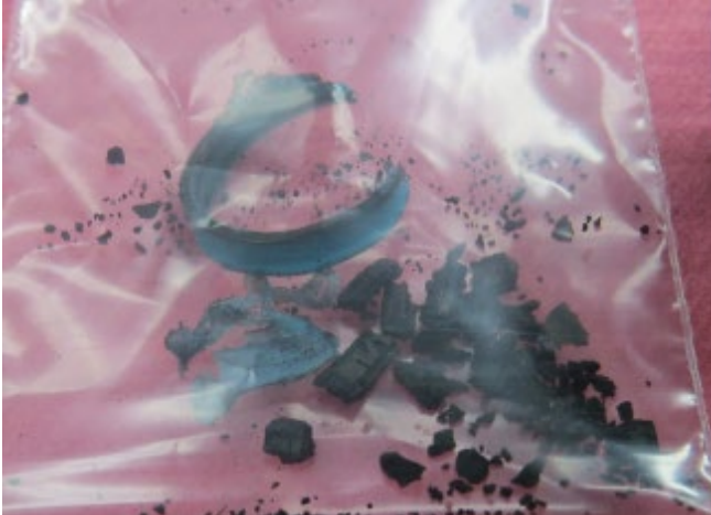
Figure 15. Primary seal, seal 5. Teflon seal and carbonized o-ring fragments.
