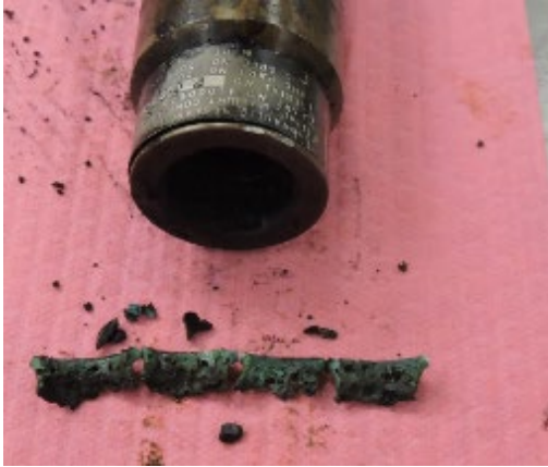
Figure 3. Cylinder gland scraper seal (seal 1) stretched out, and carbonized o-ring fragments.
