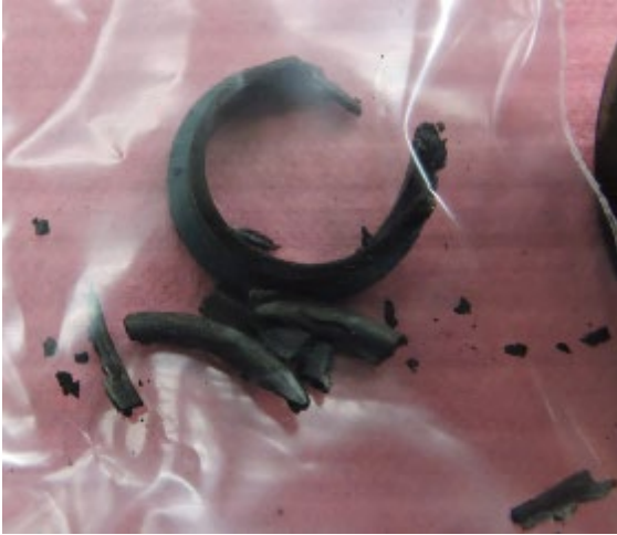
Figure 12. Seal 1, Teflon scraper seal and o-ring fragments.
