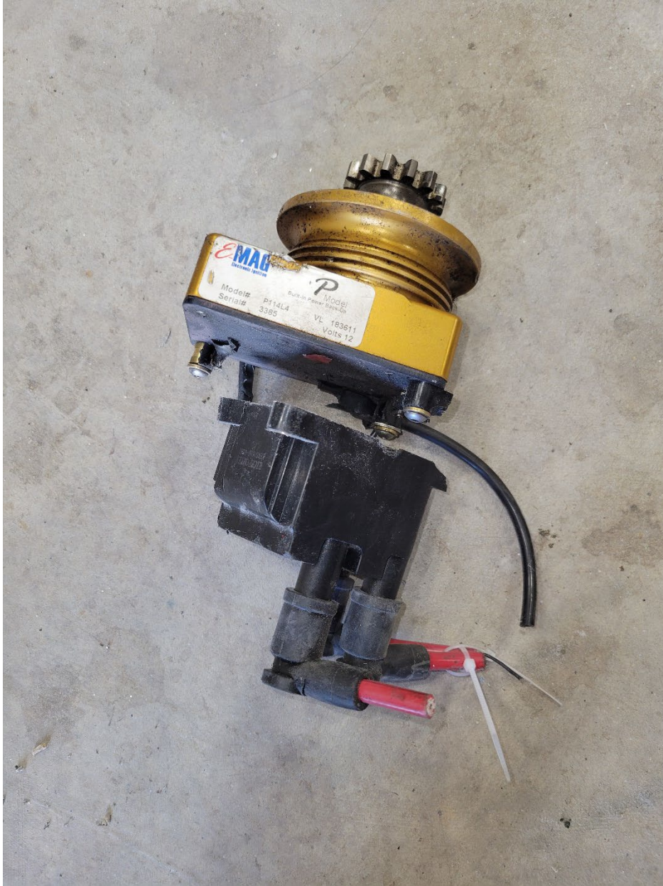
Figure 3. E-Mag ignition system removed from the accident airplane. (NTSB Photo)
