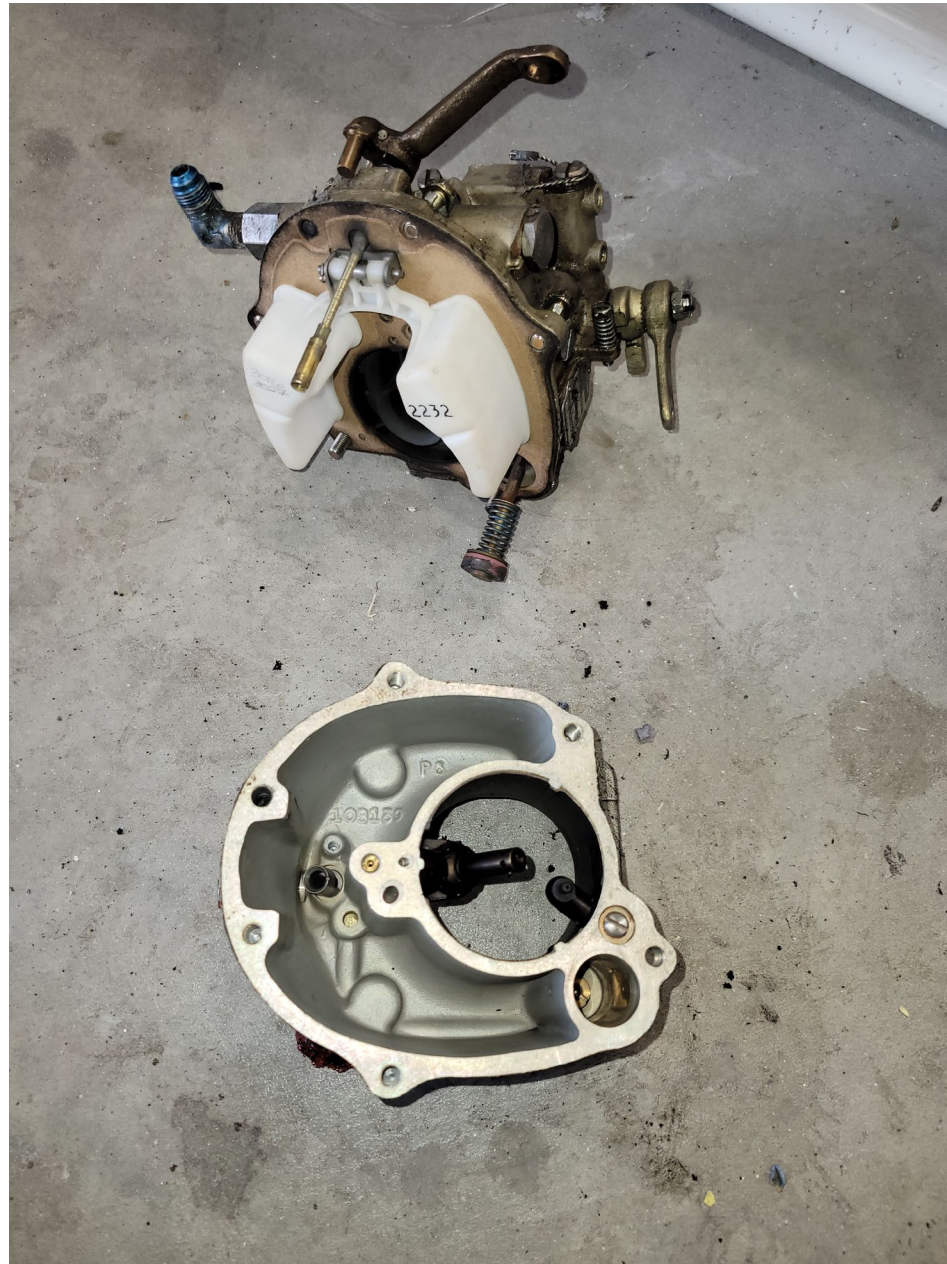
Photo 8 – Carburetor during examination (NTSB Photo)
