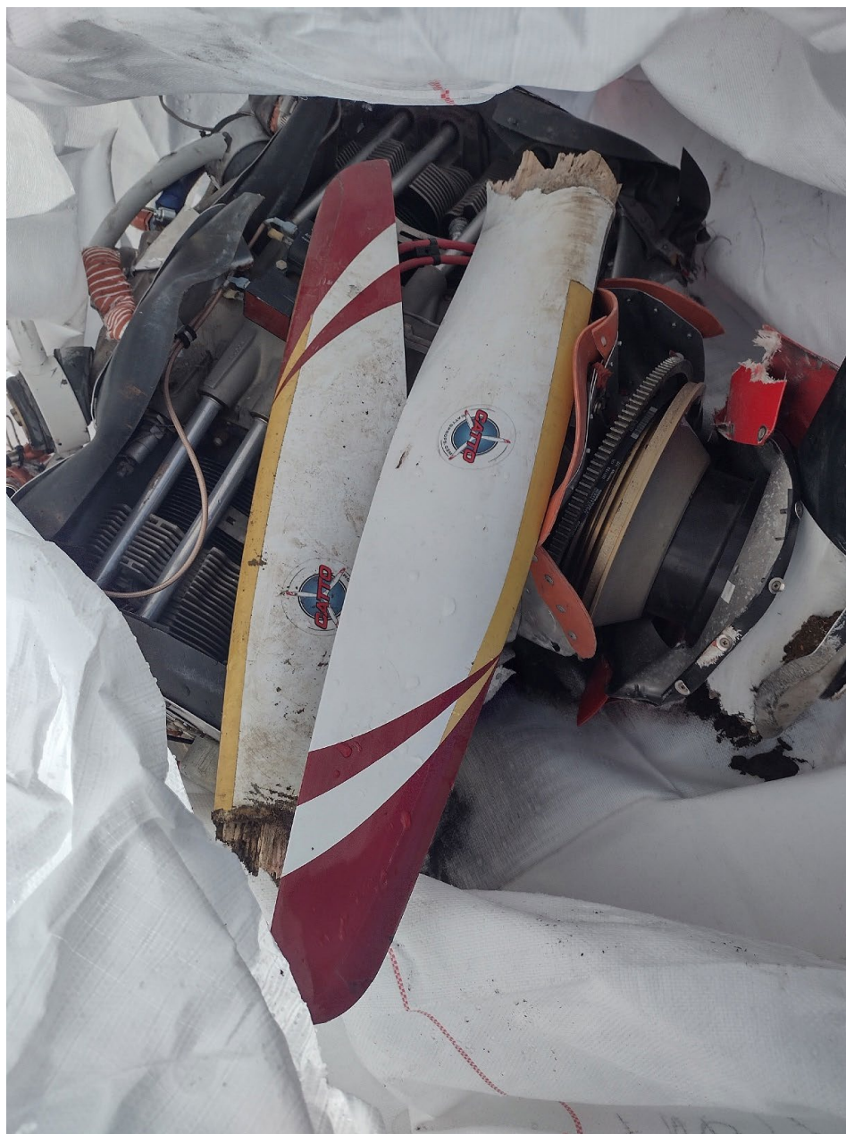
Photo 7 – Separated prop blades (Photo courtesy of AMF Aviation)
