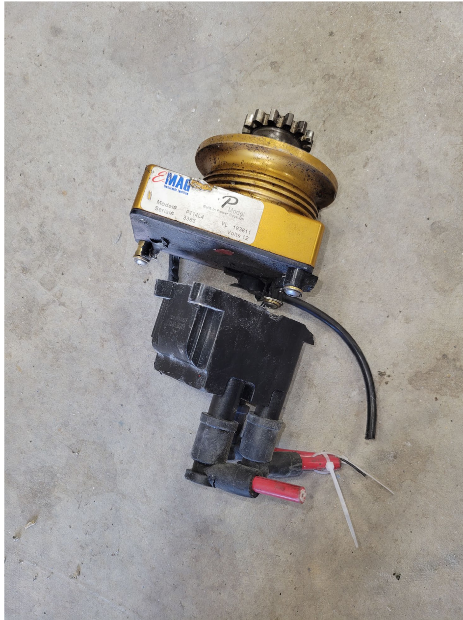
Photo 9 – E-Mag ignition during examination (NTSB Photo)
