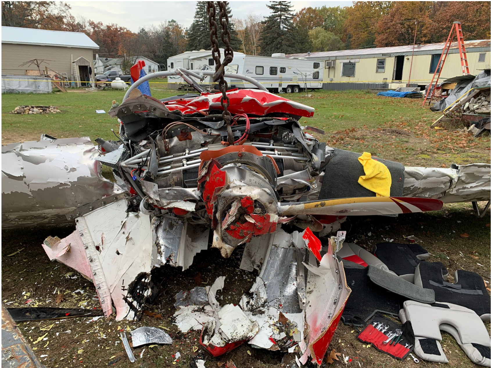
Photo 6 – View showing one prop blade intact (NTSB Photo)
