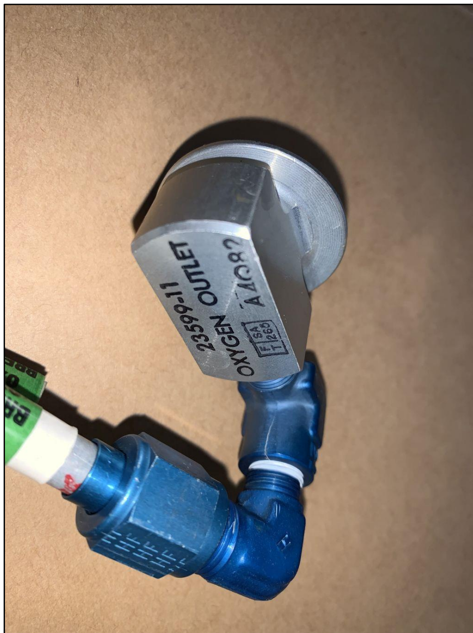
Photo 6 – Pilot-Side Oxygen Line
