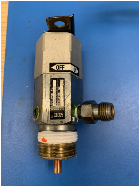
Figure 2 – Cylinder Valve/Regulator Assy (As Removed from Cylinder)
