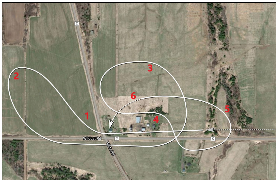
Figure 3. The airplane’s estimated ground track in the minutes before the accident, with red numbers indicating where the bank angles were measured during each turn
