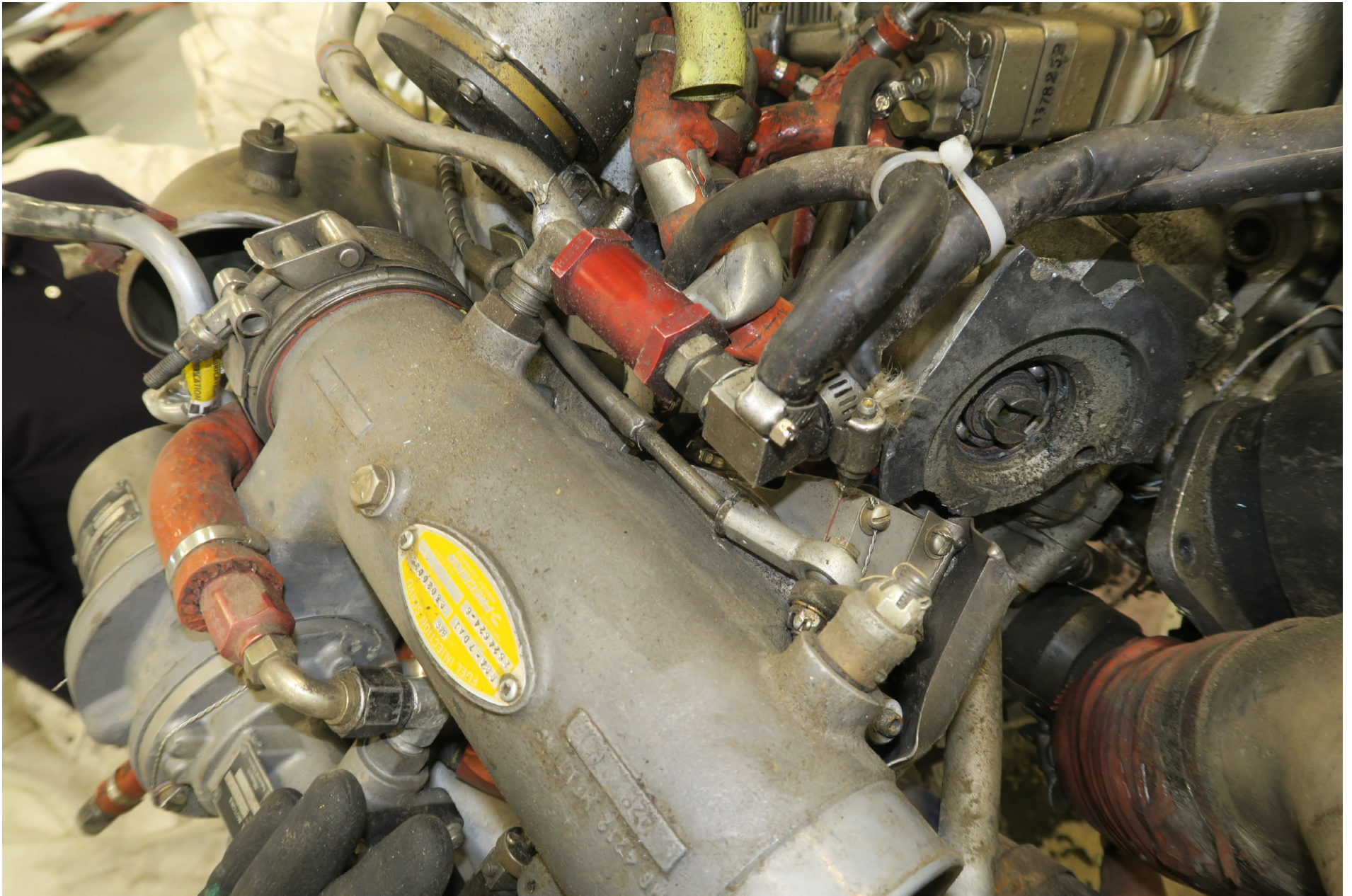
Photo 14 – Right Engine Throttle and Control Assembly
