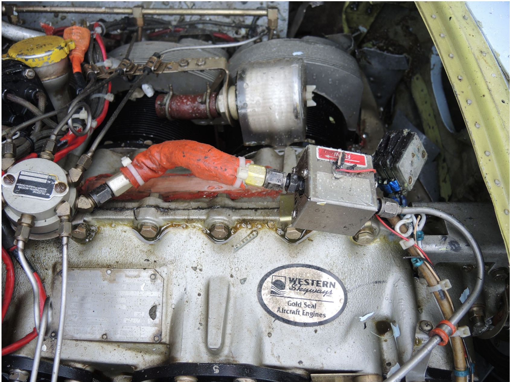
Photo 9 – Oil on Right Engine at Accident Site
