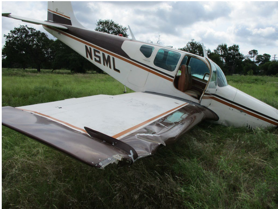
Figure 2: Damage to Right Wing
