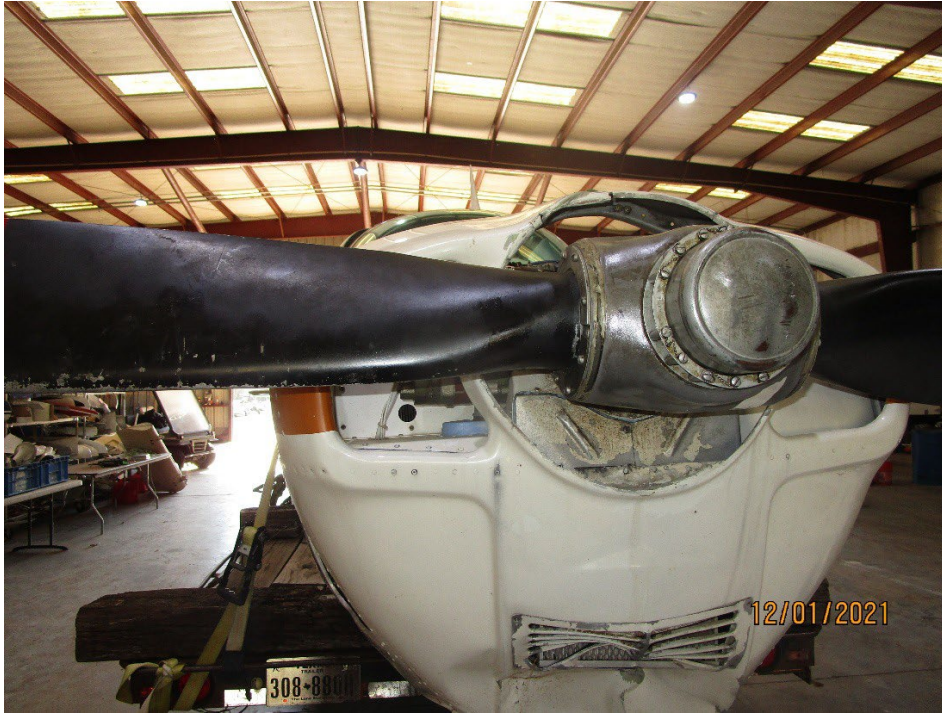
Figure 3: 2 bladed – constant-speed replacement propeller installed
