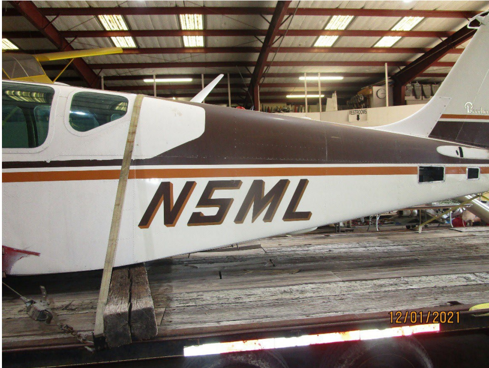
Figure 1: fuselage strapped down to trailer for engine run
