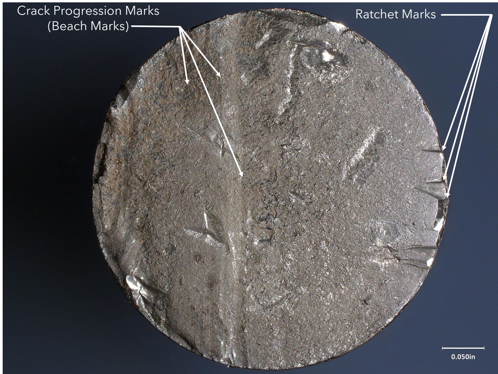
Photo 5 - Exhaust Valve Stem Fracture Surface (NTSB Photo)
