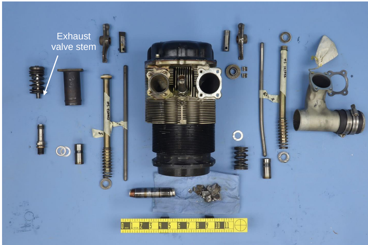
Figure 1: Number 2 cylinder assembly and ancillary components, as received. Exhaust-related components are to the left of the cylinder and intake-related components are to the right of the cylinder.
