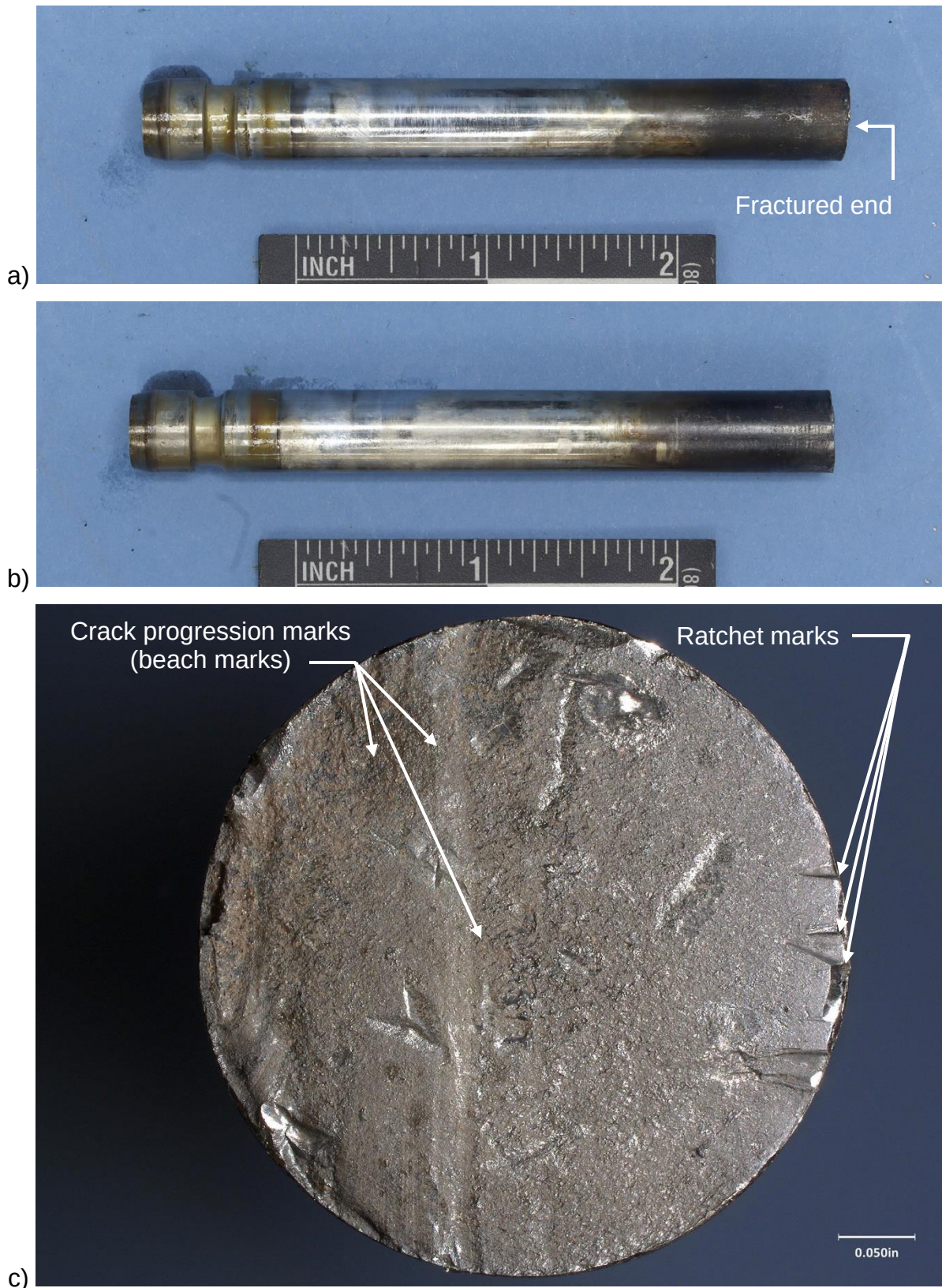
Figure 4: Images of the number 2 exhaust valve stem; a) one side of the stem; b) the other side of the stem; c) the stem fracture surface;
