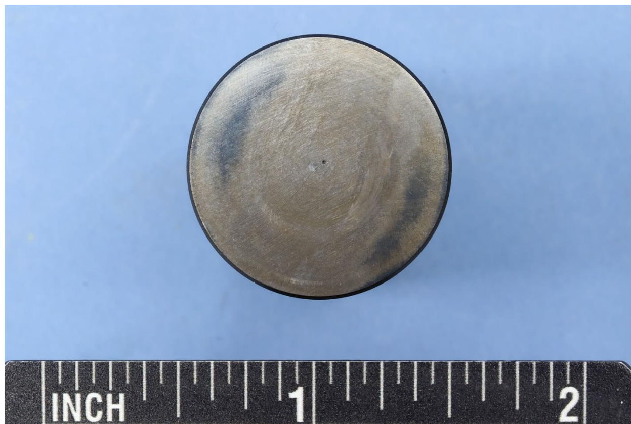
Figure 7: Image of the number 2 intake valve lifter body end face. There were no apparent smeared metal features.
