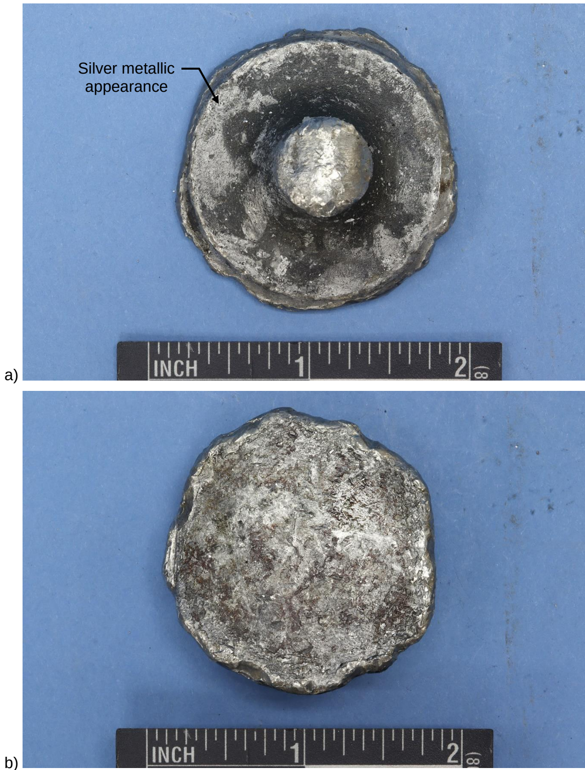
Figure 5: a) Image of the valve head fillet region and smeared fracture at the fillet to stem transition; b) image of the combustion chamber-facing side of the head; and
