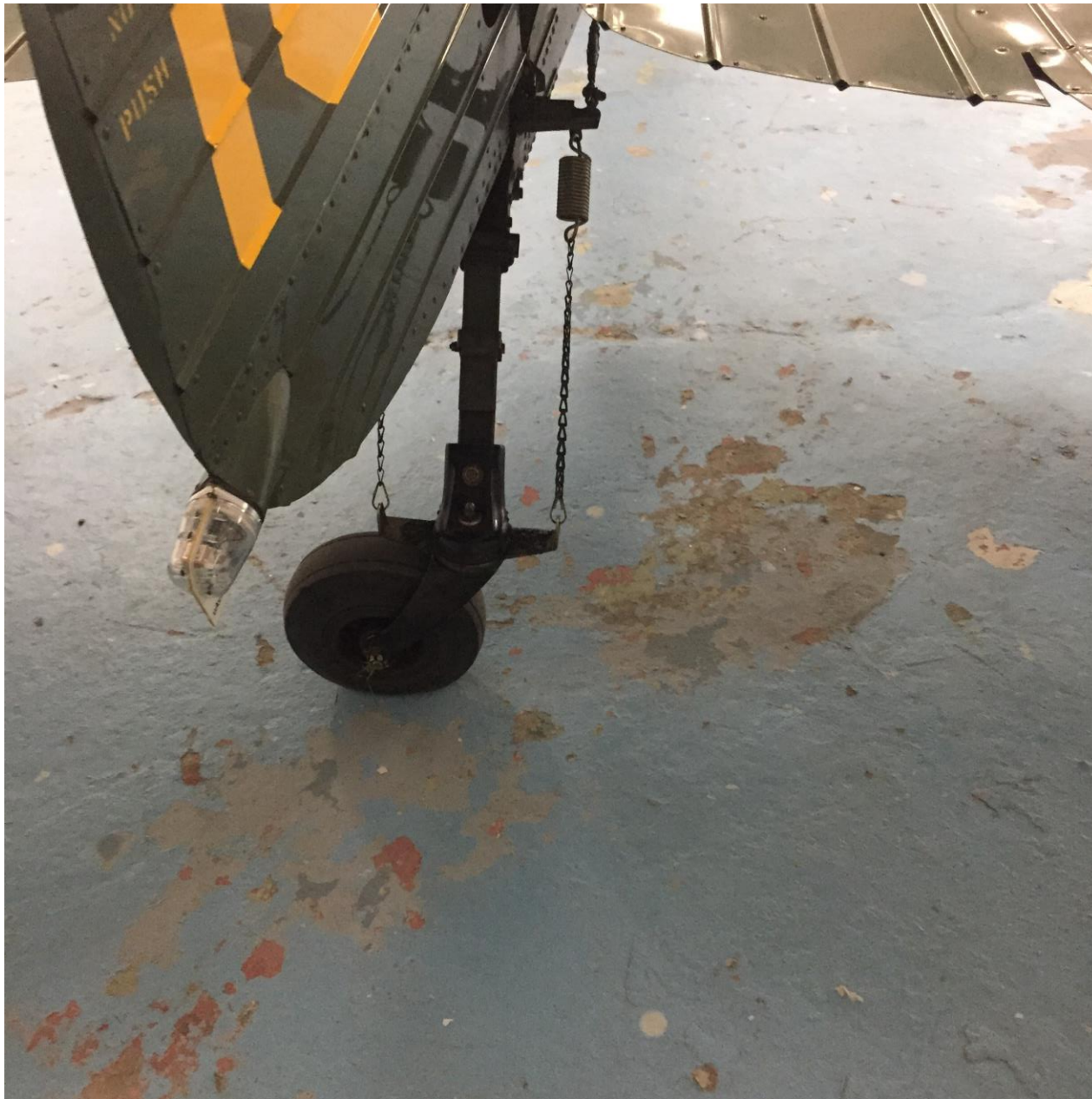
Photo 4 – Close up rear view of the tailwheel (courtesy of the Federal Aviation Administration).
