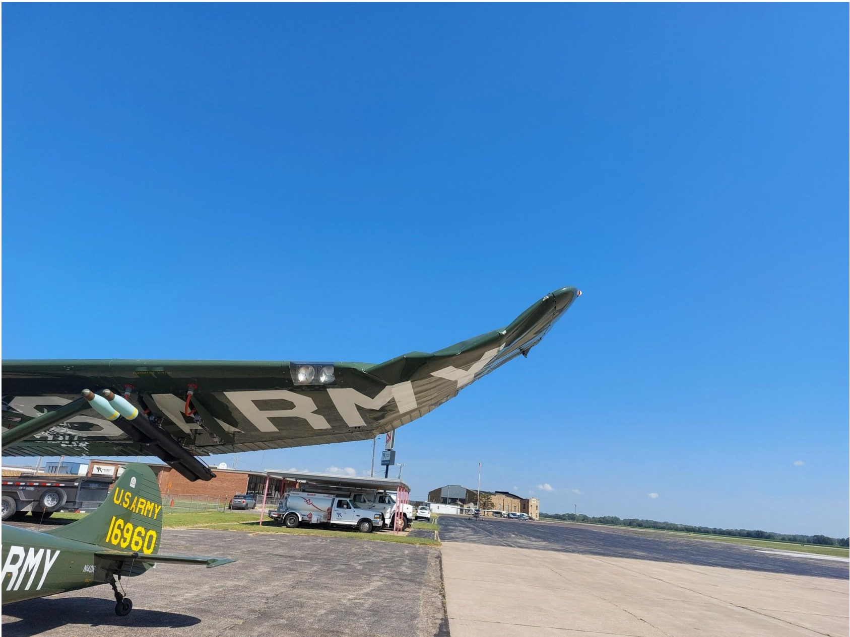
Photo 2 – Close up front view of the substantial damage sustained to the left wing after the accident (courtesy of the Federal Aviation Administration).
