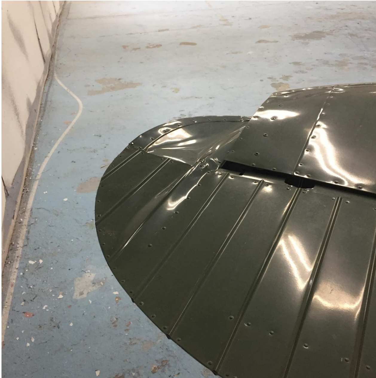
Photo 3 – Close up rear view of the substantial damage sustained to the left elevator (courtesy of the Federal Aviation Administration).
