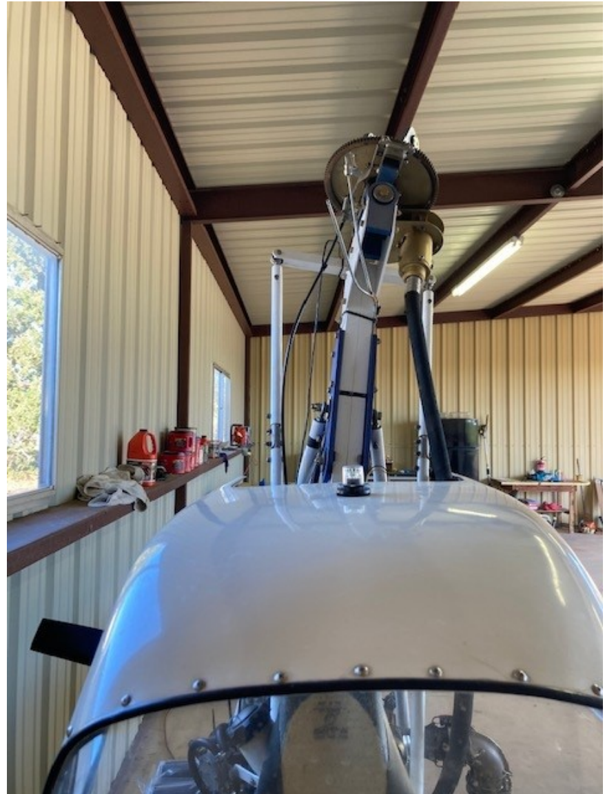
Figure 4: Damage to the Rotor Mast
