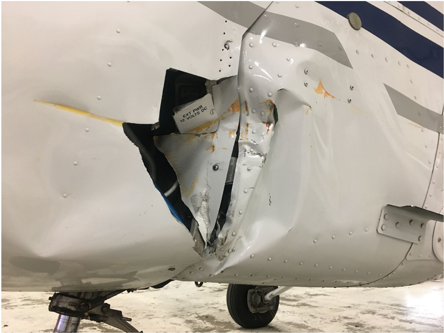
Photo of Damaged Fuselage, Courtesy of FAA
