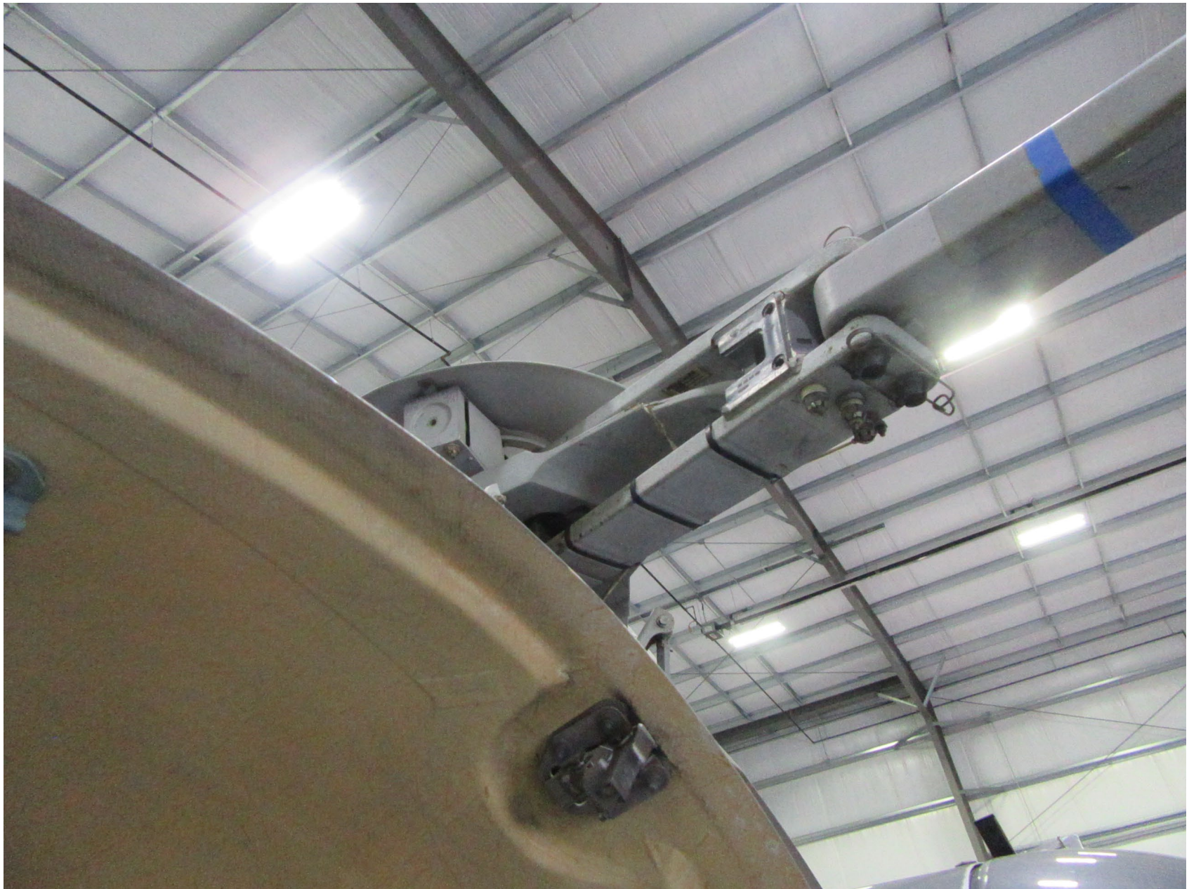
Photo 1 – Blue Main Rotor Blade Starflex Fracture
