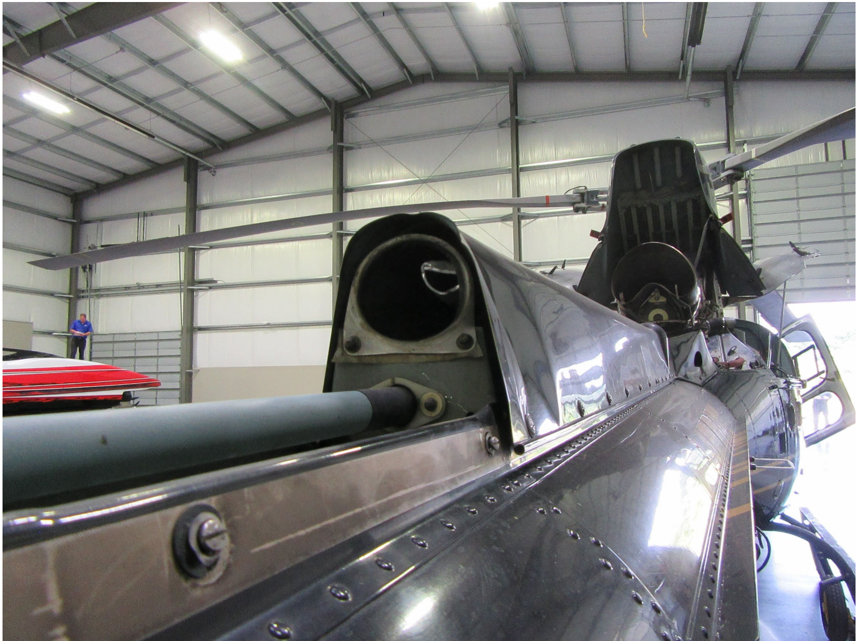
Photo 3 – Fractured Tail Rotor Driveshaft
