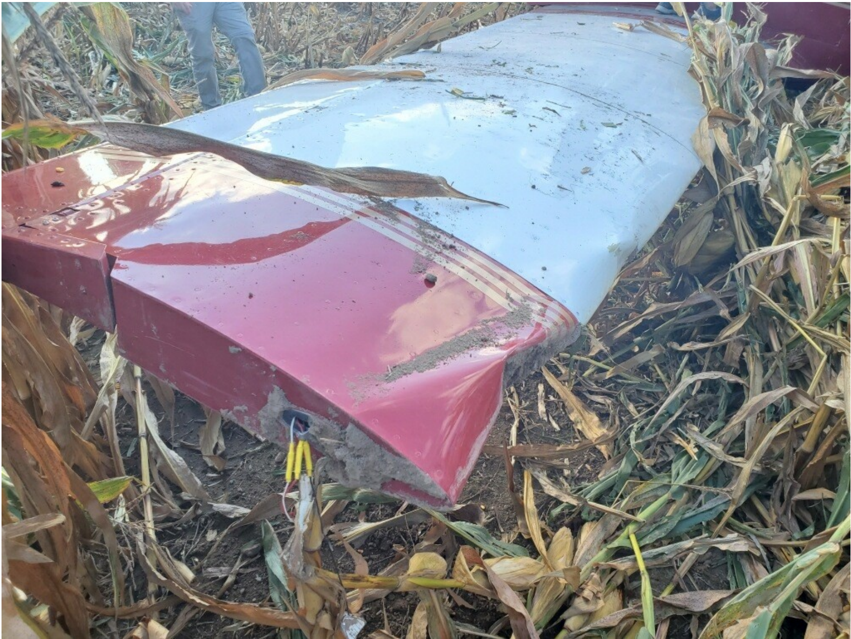
Photo 2 – Damage to Left Wing (Photo from FAA)
