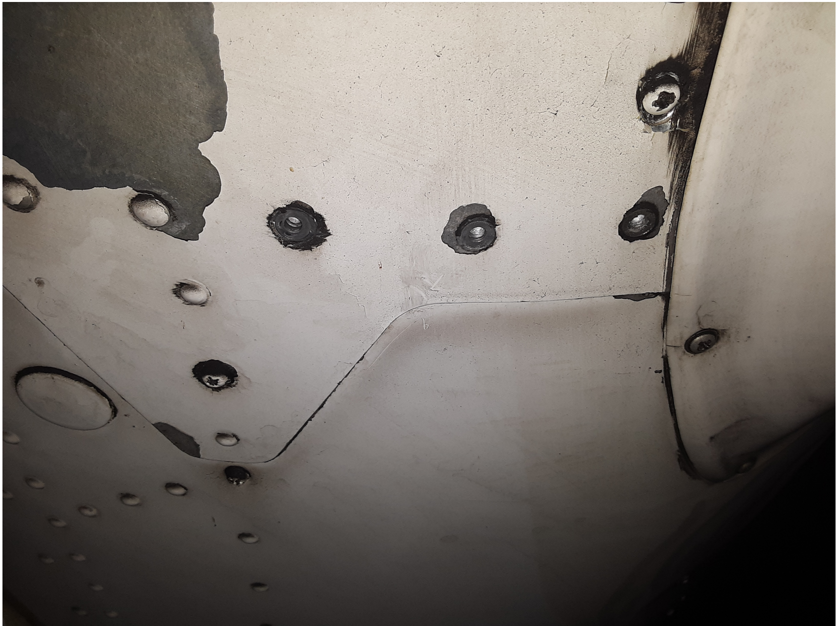
Photo 3 – Closeup of Popped Rivets in Lower Part of Fuselage (Source: Kent State)
