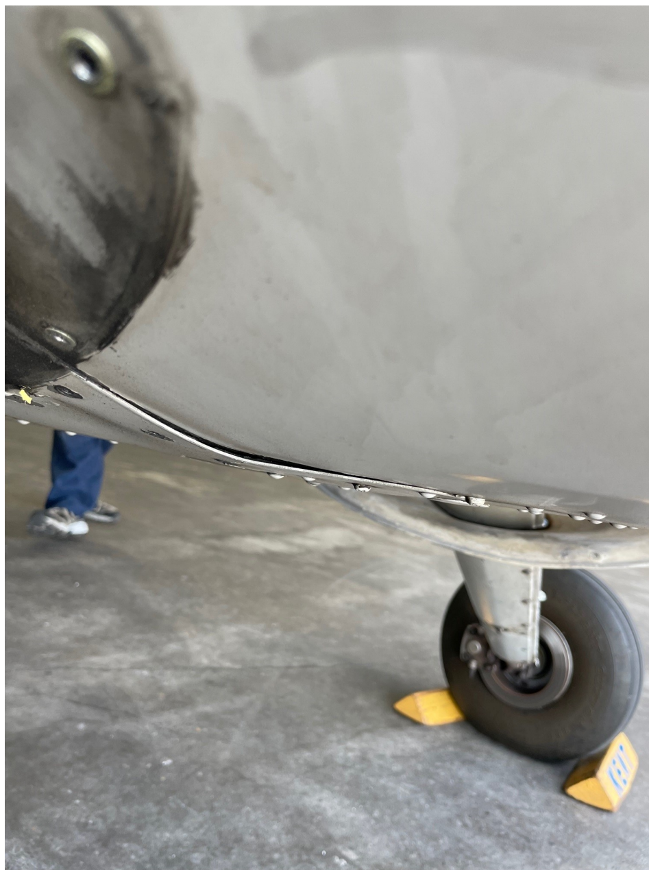
Photo 1 – Lower Part of Fuselage Buckled (Source: Kent State)
