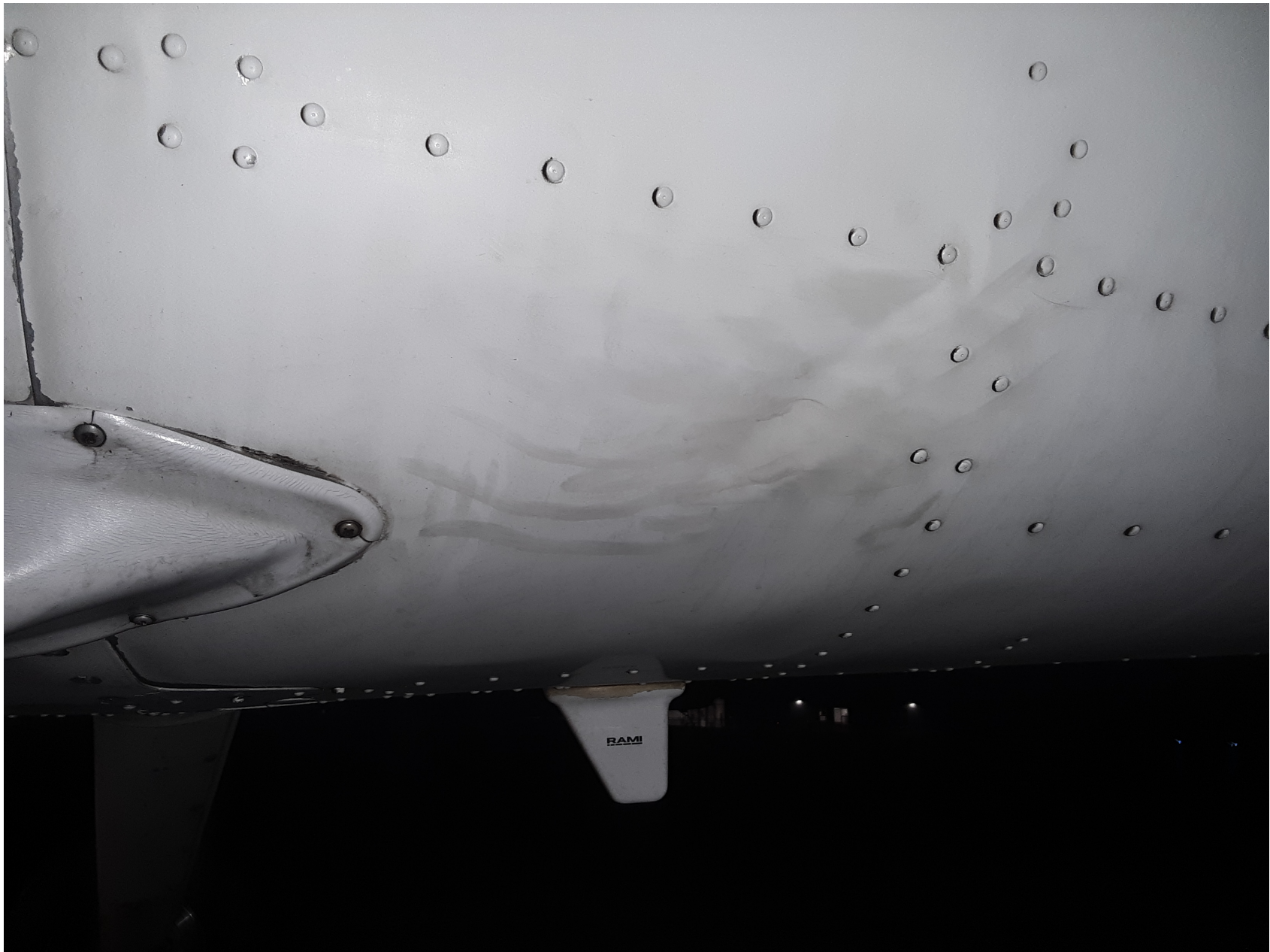
Photo 2 – Wrinkles in Lower Part of Fuselage (Source: Kent State)
