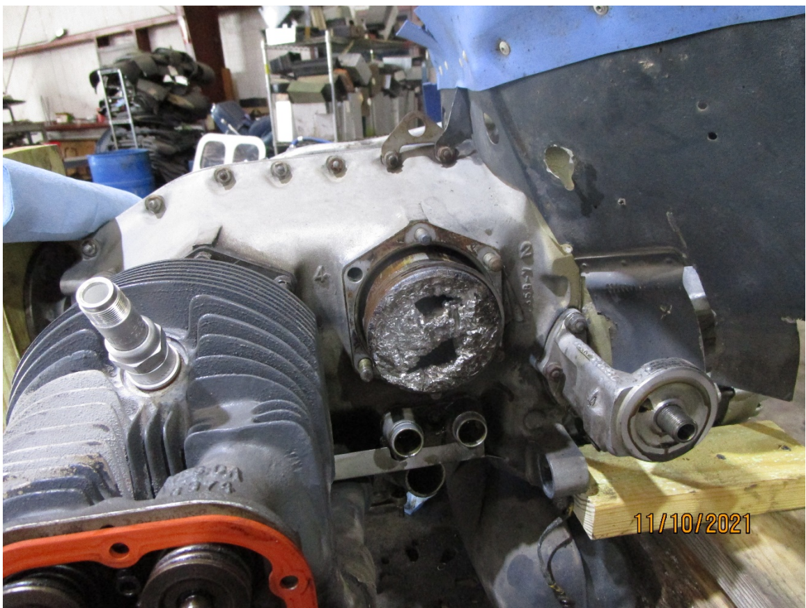
Engine, with cylinder separated: note damage to the piston.
