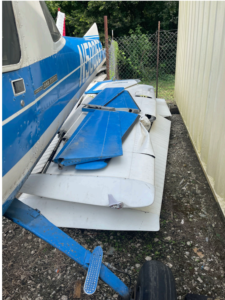
Photo 1 – Damaged Left Wing
