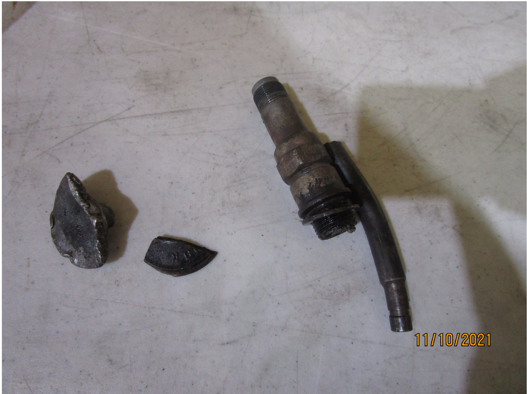
Photo 4 – Broken Exhaust Valve
