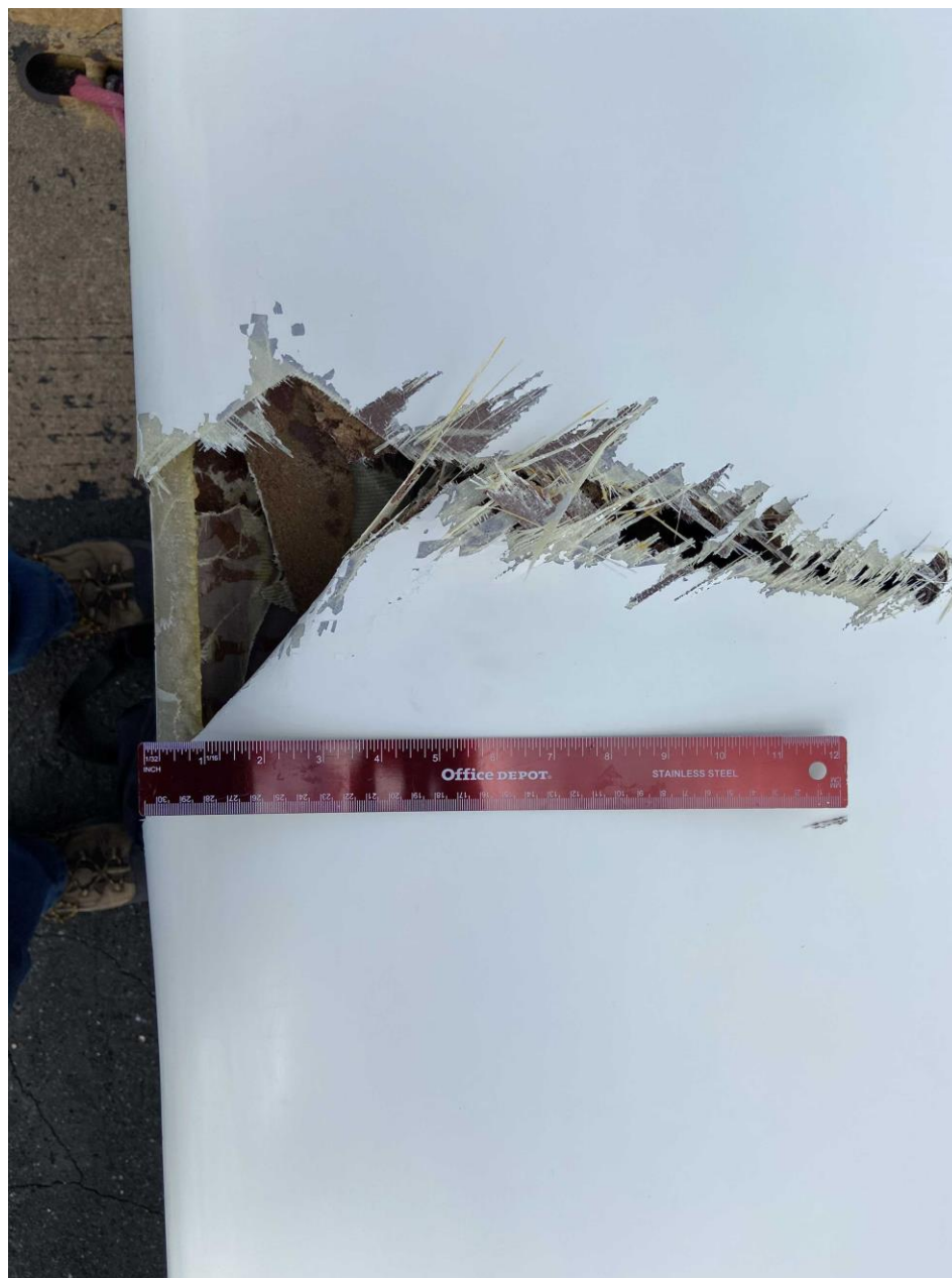
Photo 3 – Left Wing Damage (Photo Provided by Federal Aviation Administration)
