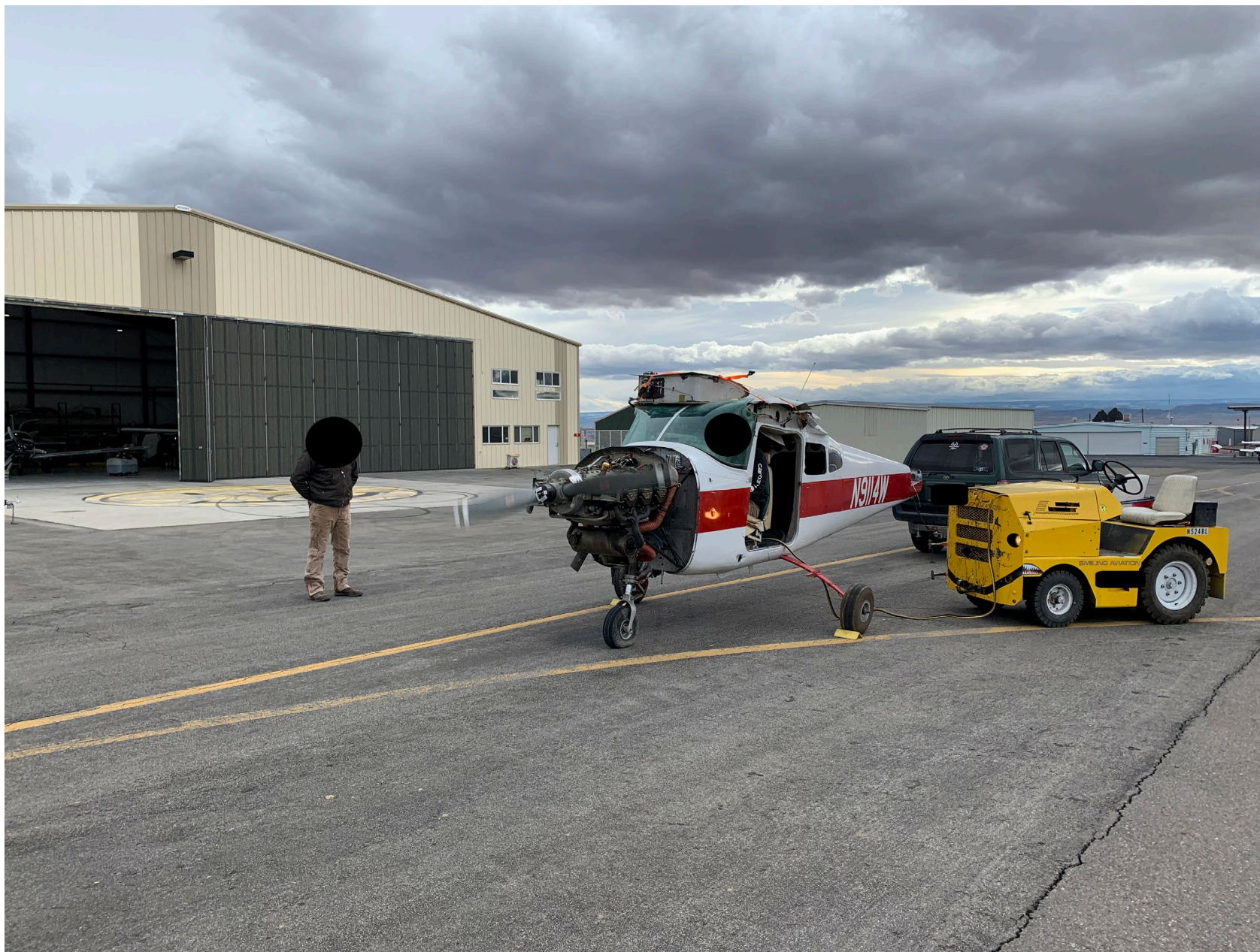
Photo 12 – View of the engine operating during the test run.
