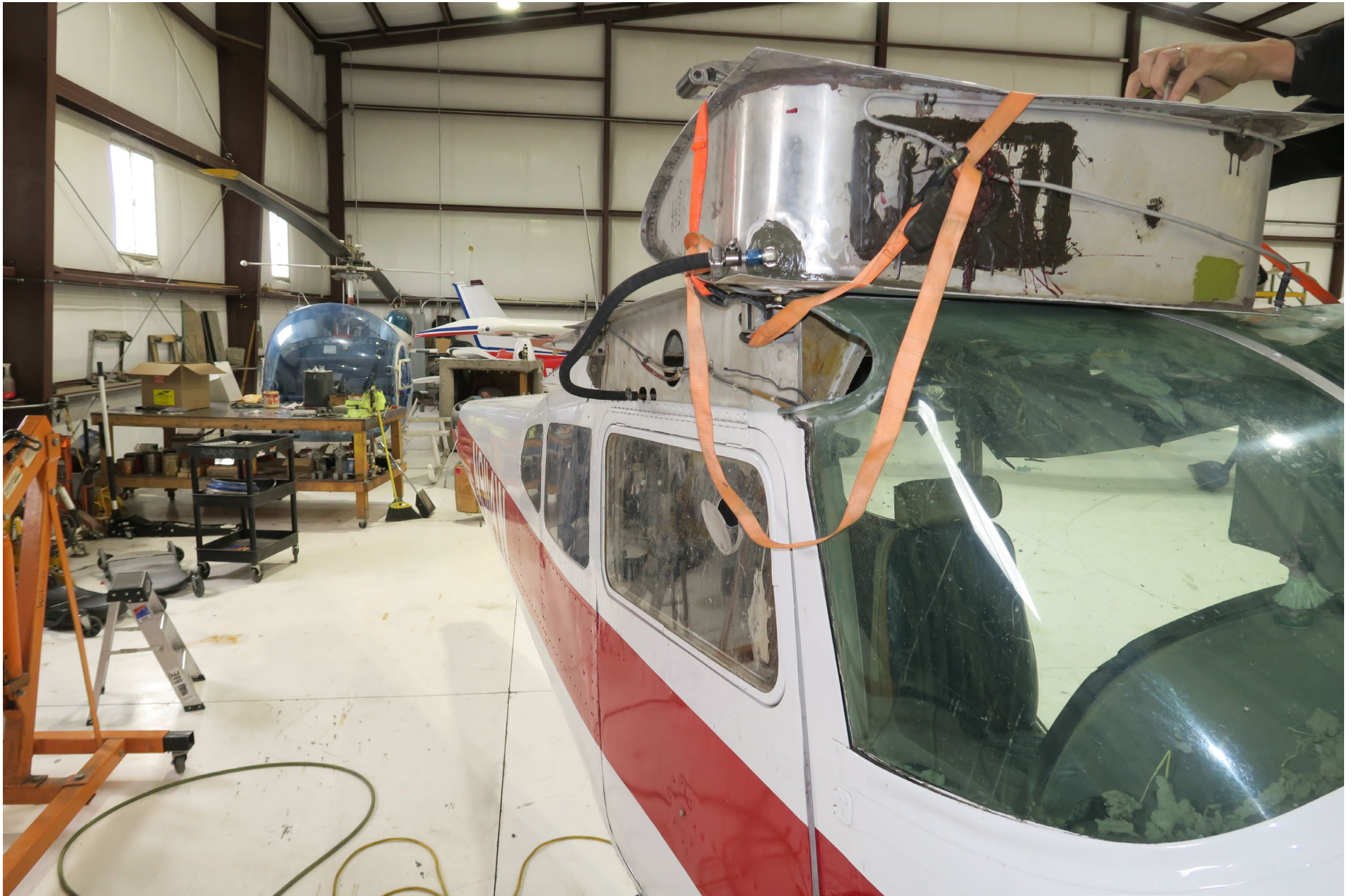
Photo 9 – View of the fuel tank mounted on the fuselage and connected to the fuel system (courtesy of Textron Aviation).
