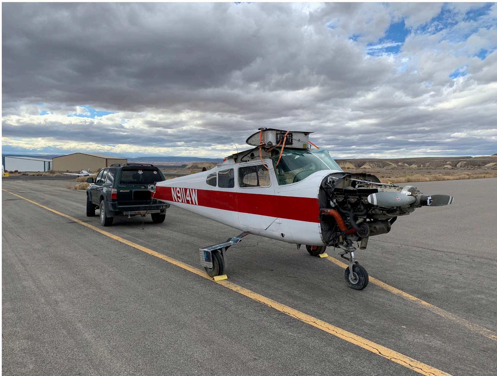
Photo 11 – View of the airplane setup for an engine test run.
