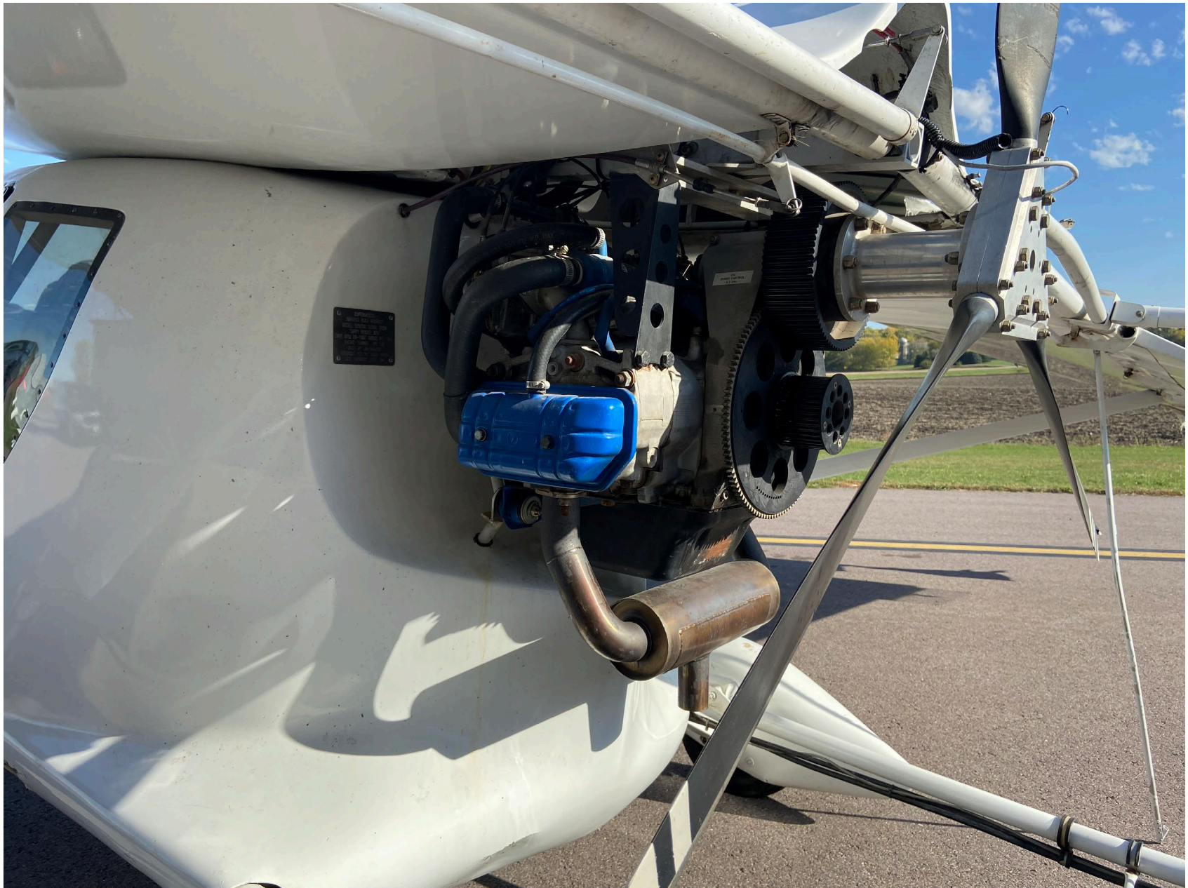
Photo 3 – Engine with no drive belt (Courtesy of FAA)
