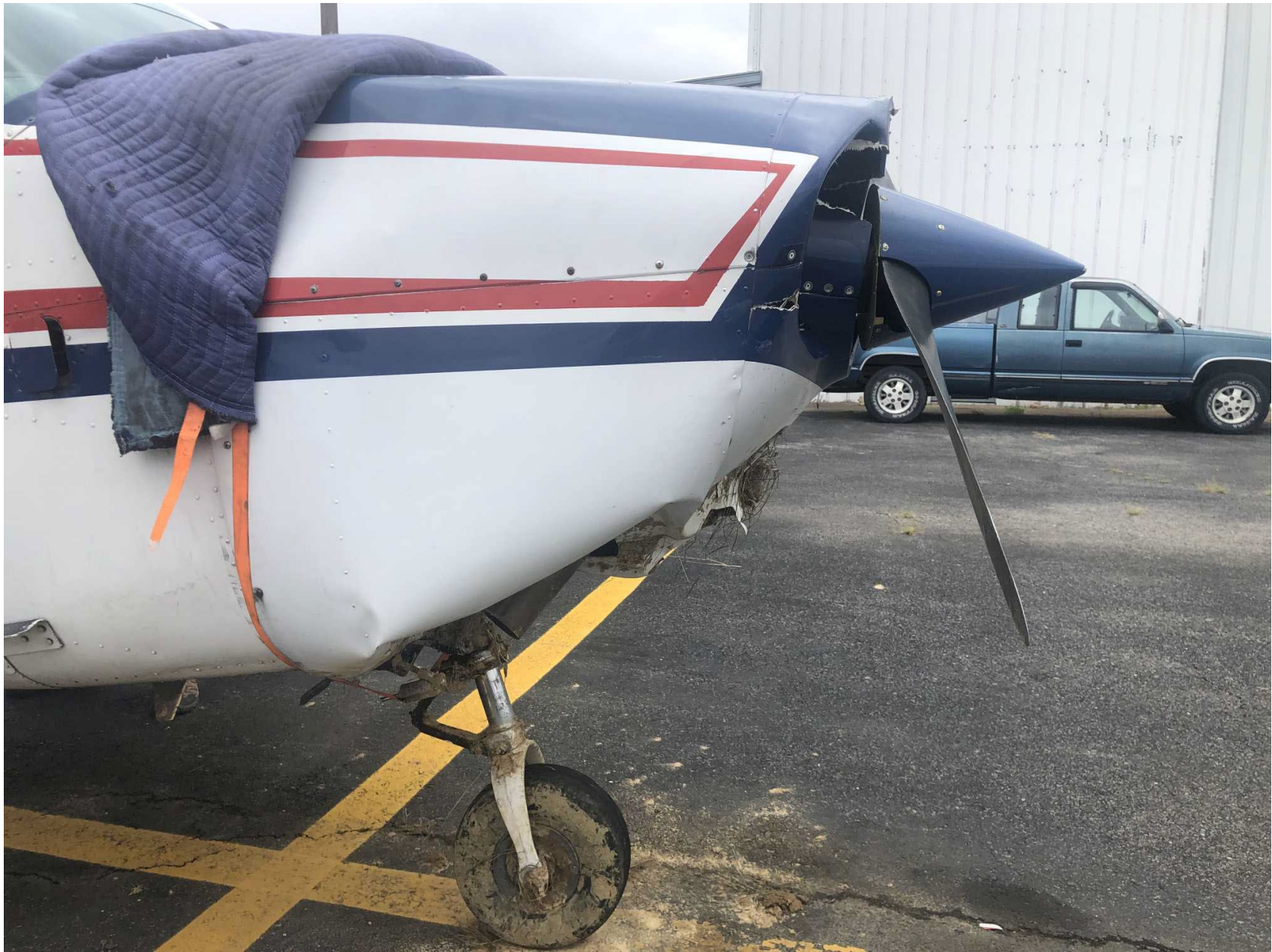
Photo 1 – View of airplane showing engine sagging (FAA photo)
