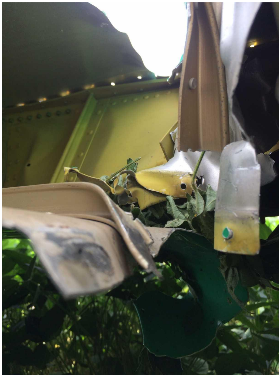
Photo 3 – Left Wing Spar Damage (Photo Provided By Pilot)
