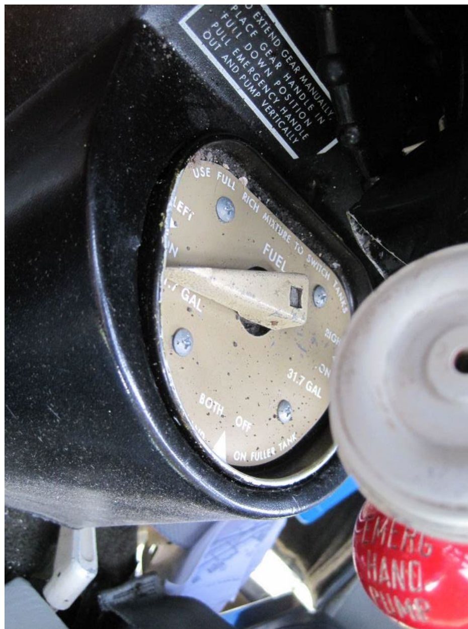
Photo 3 – Fuel Selector (FAA Photo)
