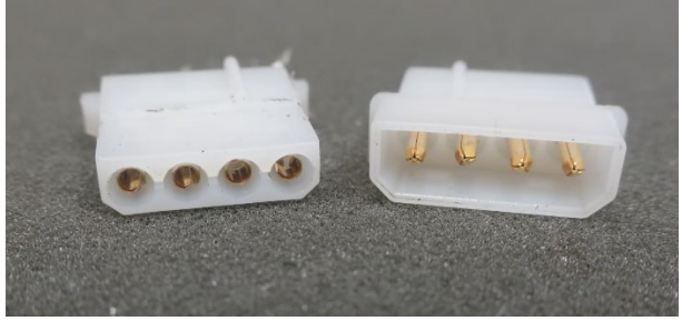
Figure 5. Female and male halves of the rpm signal cable connector.
