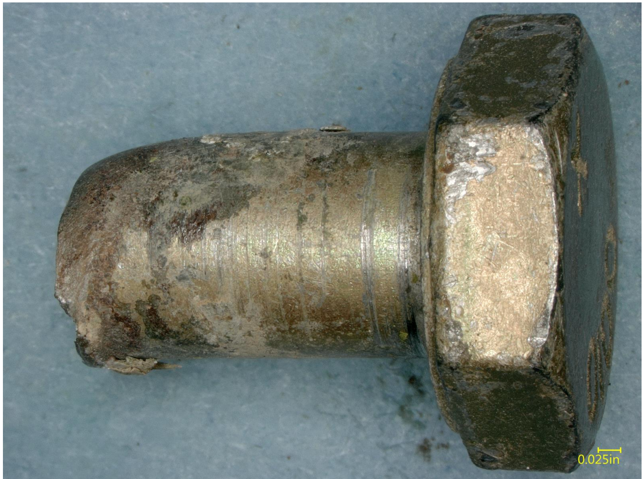
Figure 7 – Side view of the bottom outboard bolt remnant.
