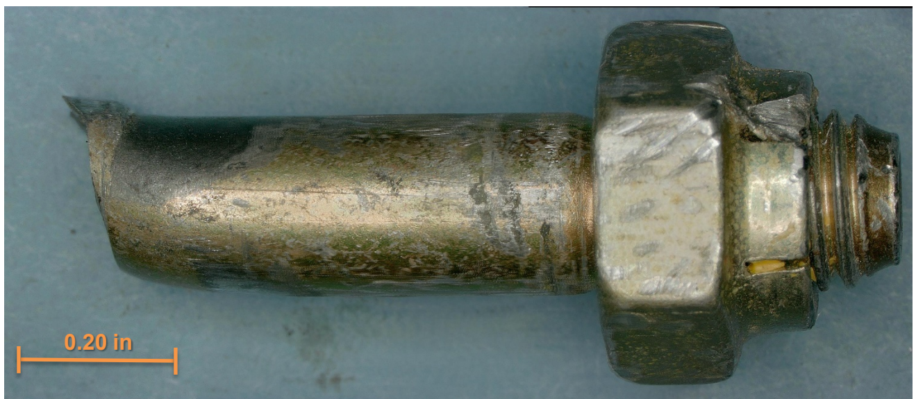
Figure 8 – Side view of the top outboard bolt remnant.
