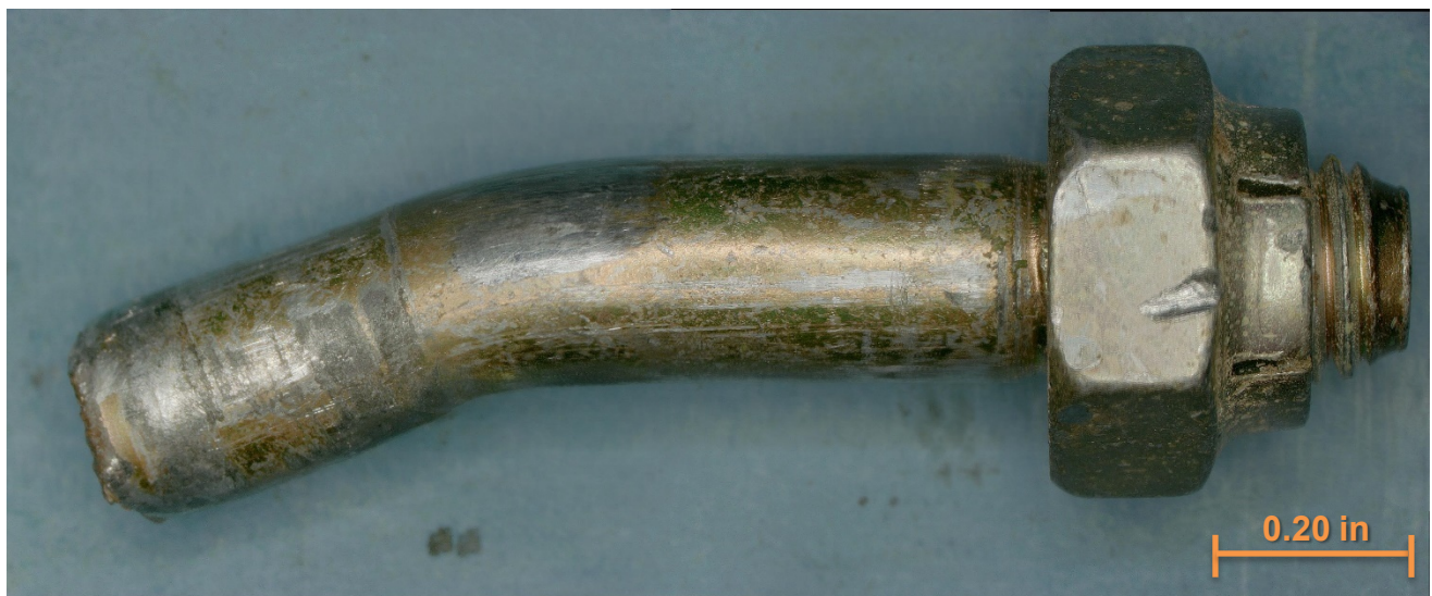
Figure 12 – Side view of the top bolt remnant, second from outboard.
