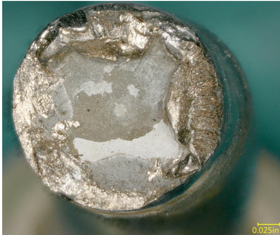
Figure 13 – View of the fracture surface of the top bolt remnant, second from outboard.
