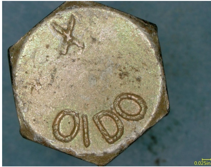
Figure 3 – The head markings on the bottom inboard bolt remnant.
