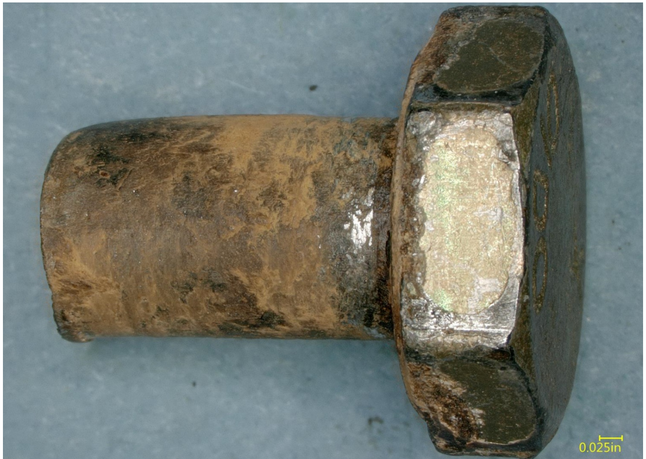
Figure 2 – Side view of the bottom inboard bolt remnant, as received.
