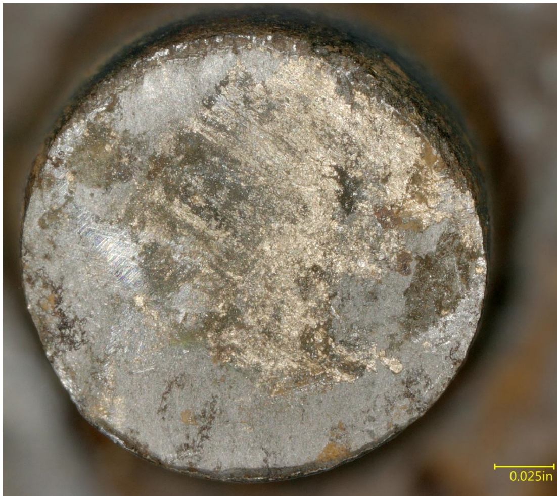
Figure 4 – Fracture surface from the inboard bottom bolt, as received.
