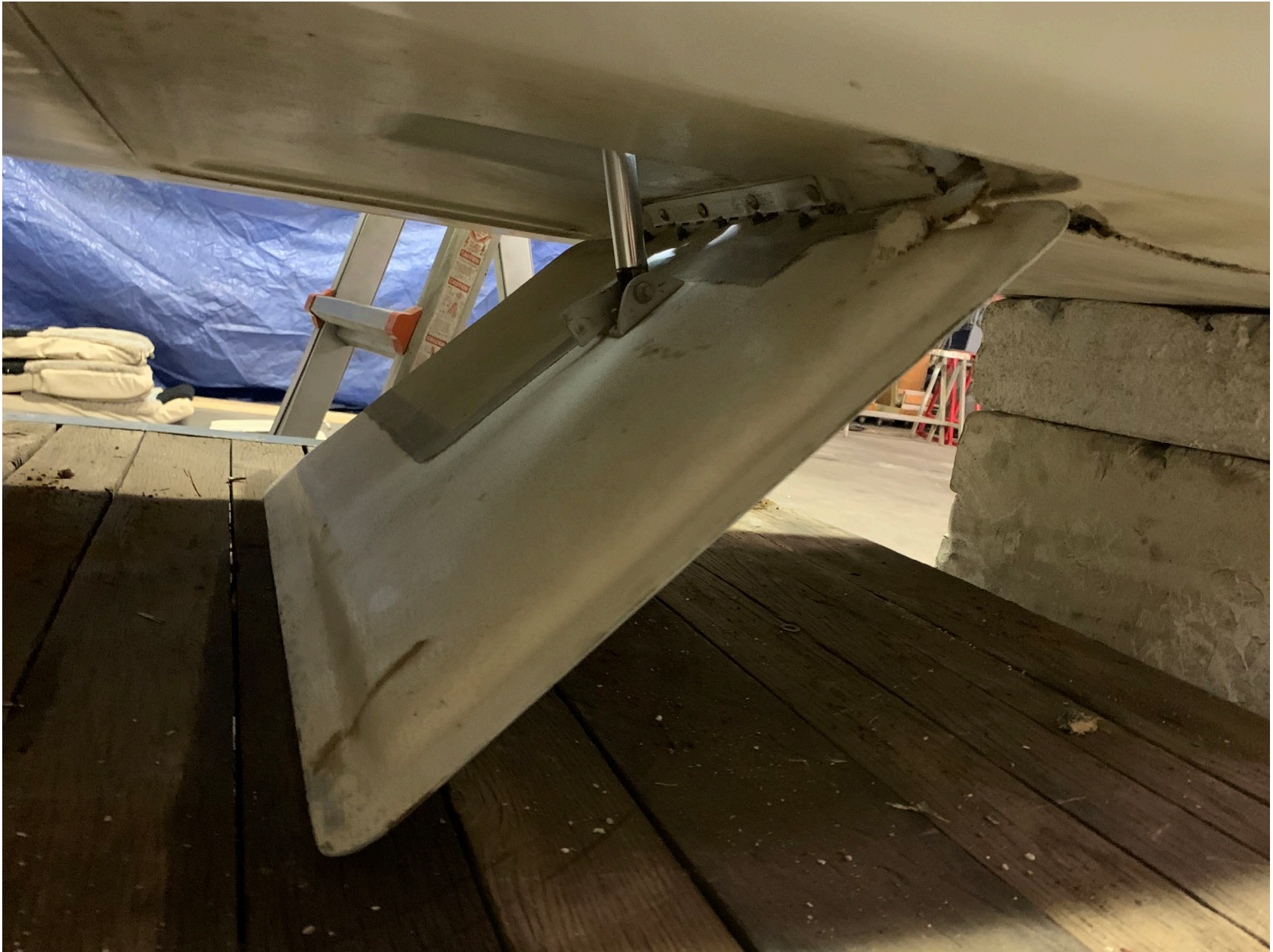
Photo 9 – View of the extended airbrake, showing the top of the panel.
