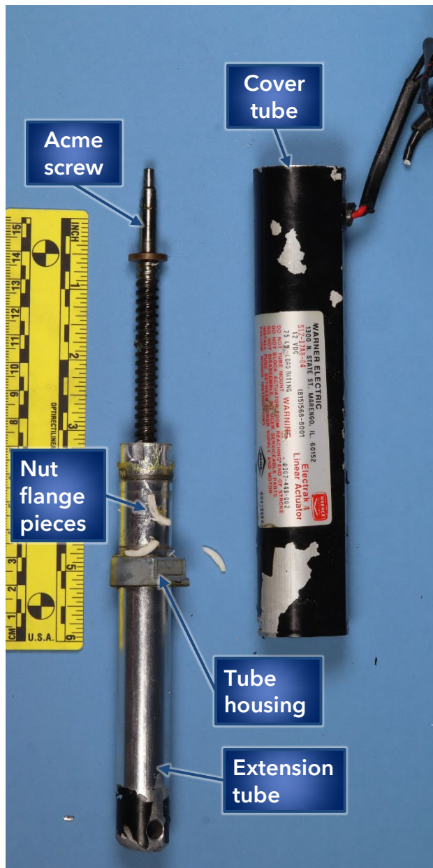
Figure 4. Linear actuator after disassembling the extension rod and acme screw from the cover tube.
