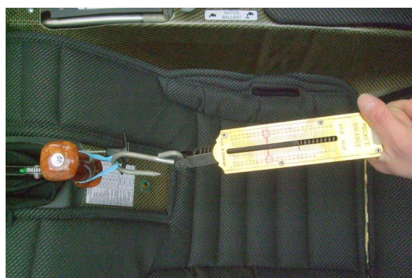
Fig. 4 Inspection of elevator control rod - apply a force to the stick
